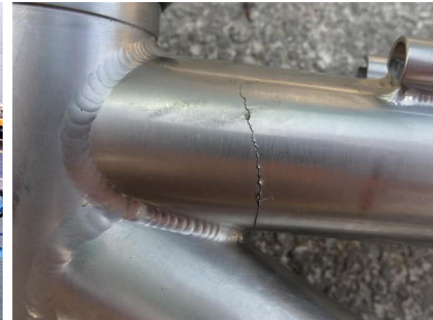
Crack on a bike frame starting from weld seam
