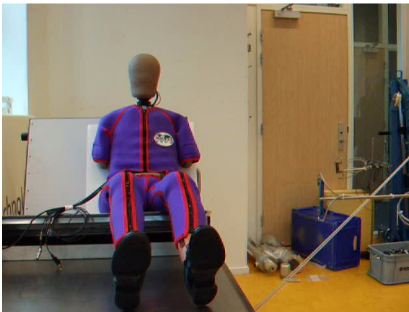
'WorldSID' pelvis prototype in 23.4 kg mass impactor test
