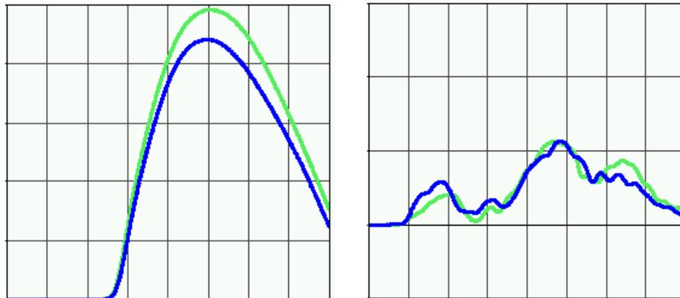
**Figure 5** Rib intrusion and upper spine acceleration of ES-2 dummy barrier height of barrier depicted in Figure 19; barrier height for green curve 20 mm higher
