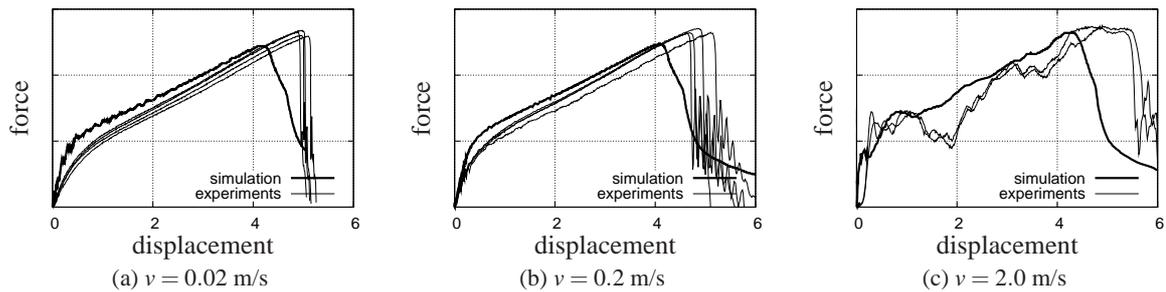
Figure 9: KS2-60°: comparison of experiments and simulation for different load speeds
