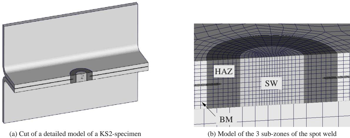
Figure 3: Detailed Model of Spot Weld
