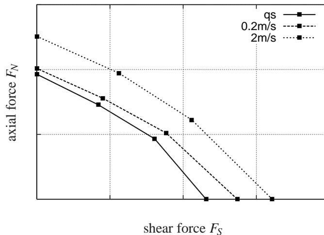
Figure 10: Critical force of DC04 dependent on the strain rate derived from the detailed spot weld model
