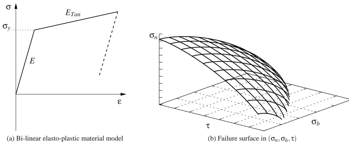
Figure 5: Material and failure model of MAT\_SPOTWELD\_DA
