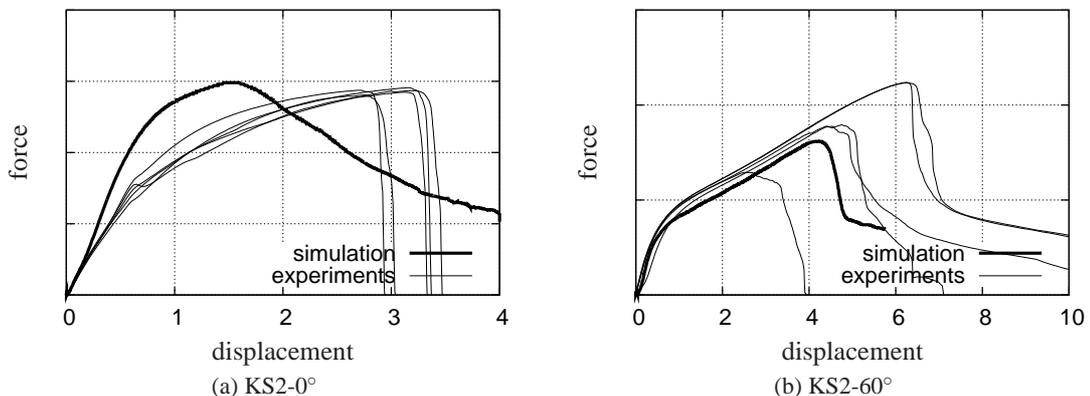
Figure 6: Comparison of the detailed model with experiments for HL320LA on coupon level
