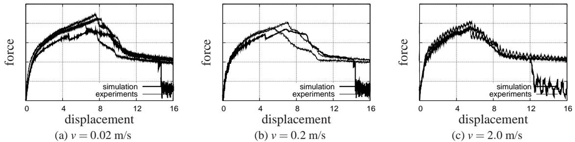
Figure 8: Coach peel: comparison of experiments and simulation for different load speeds
