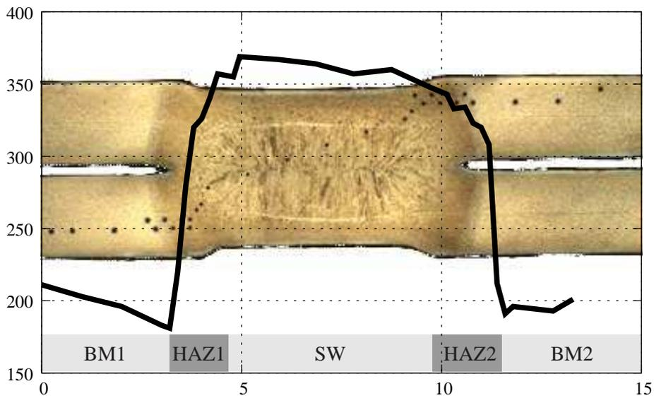
Figure 2: Cut of a spot weld (HT600XD) with corresponding Vickers hardness test
