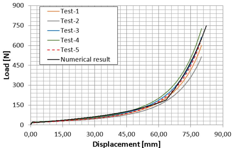
Fig.7: Experimental and numerical results of the picture frame test
