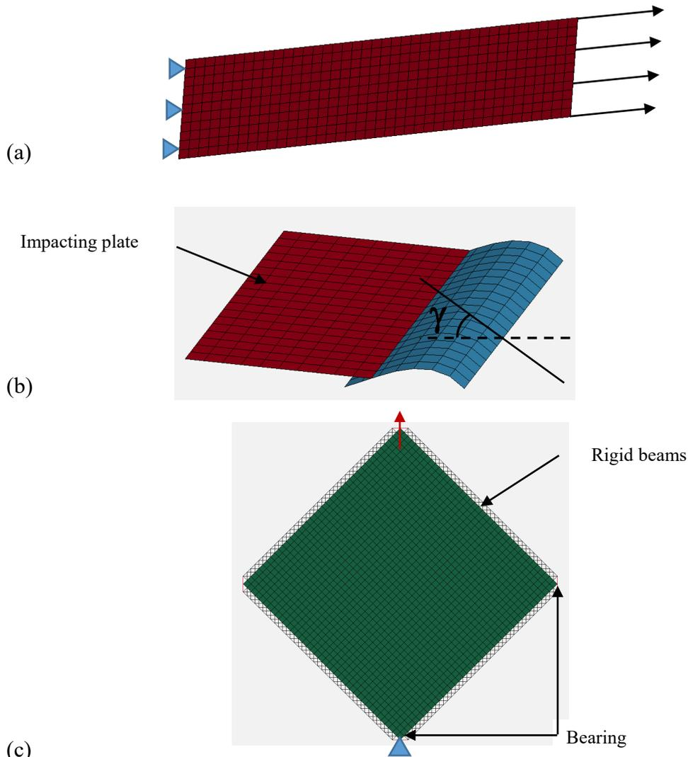
Fig.4: Employed FE model: (a) tensile test (b) Bending test and (c) picture frame test
