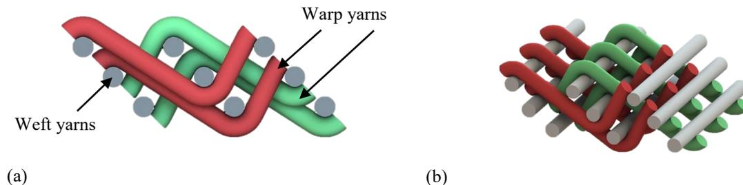
Fig.1: Fabric structure: (a) plane view and (b) tridimensional view
