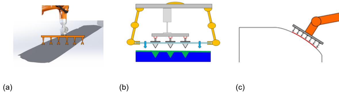
Fig.8: Automated industrial process: (a) Transport and lay-up of the fabric, (b) positioning on the forming table and (c) draping
