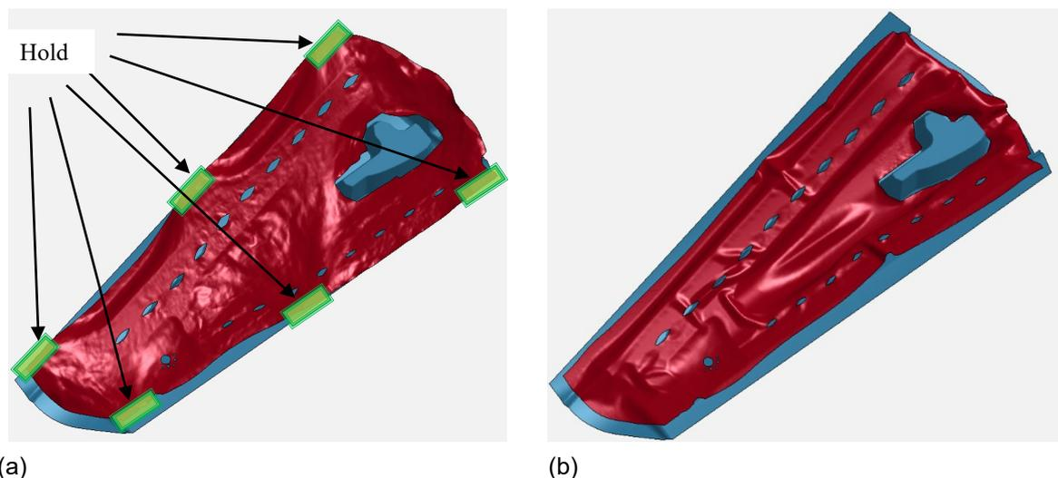
Fig.11: Final configuration of the fabric subjected to self weight loading: (a) hold by robot and (b) after lay-up on the preforming table
