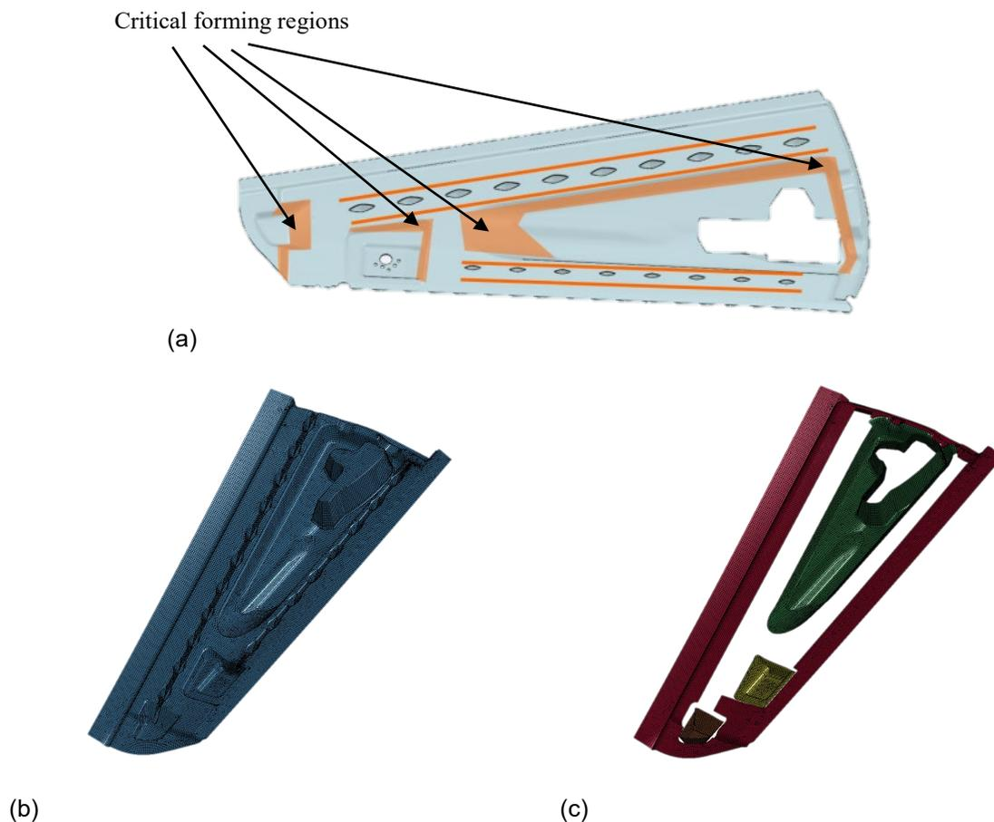
Fig.9: Employed FE model for draping simulation: (a) Critical forming regions, (b) forming table and (c) designed forming tools
