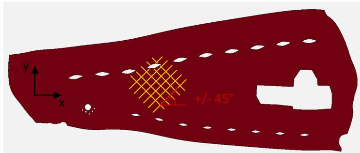
Fig.10: Assumed initial fiber orientation in the performed draping simulation
