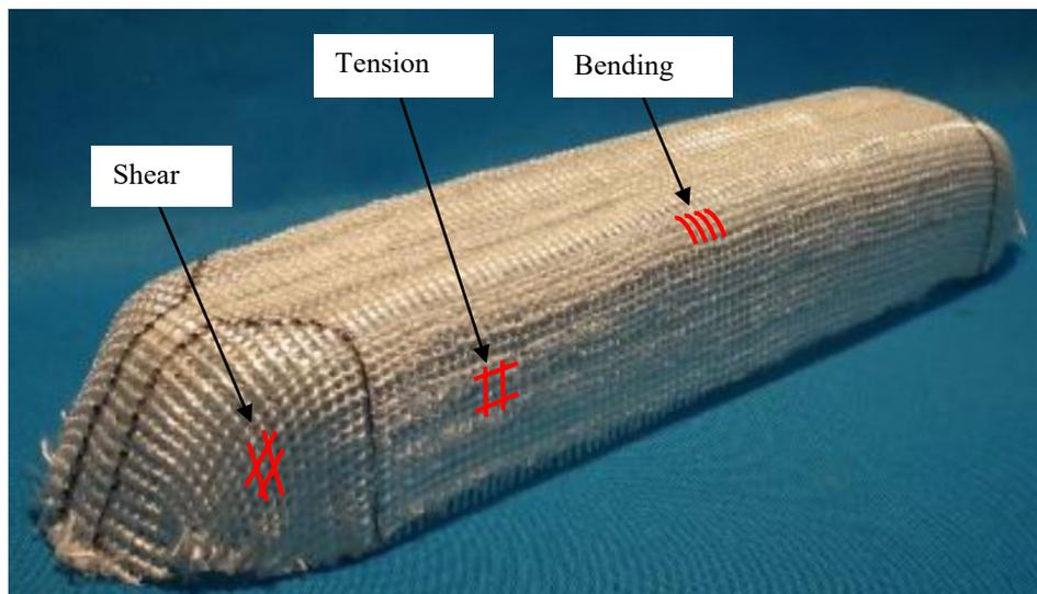
Fig.2: Observed deformations after draping for a typical geometry taken as example from the literature [3]
