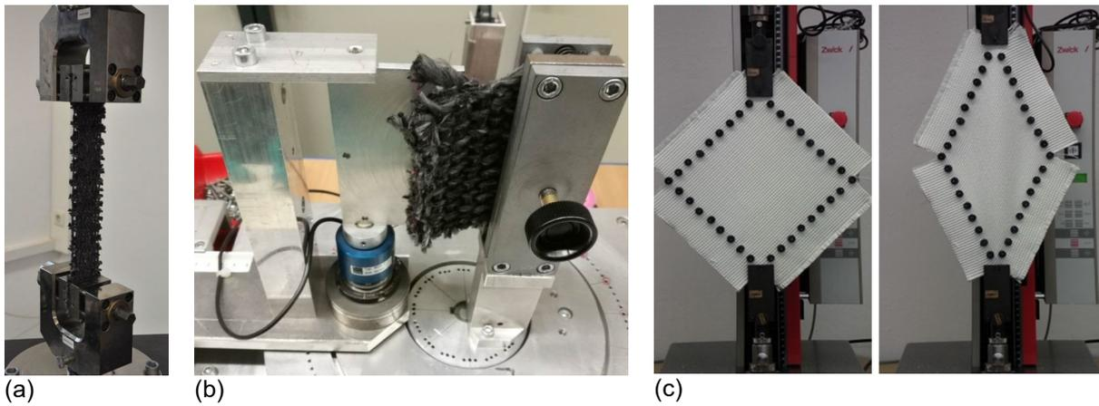
Fig.3: Experimental test set-up: (a) tensile test (b) Bending test and (c) picture frame test
