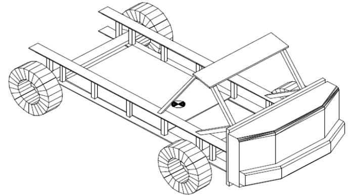
Moving Deformable Barrier (MDB)
