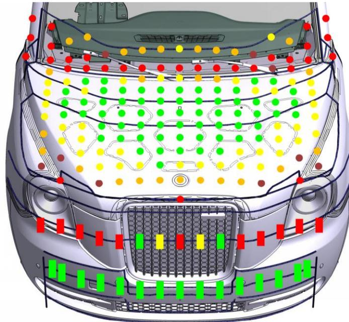
Fig.23: Pedestrian Impact Positions and Geometry Mark-Up Lines (circle head, rectangle leg)
