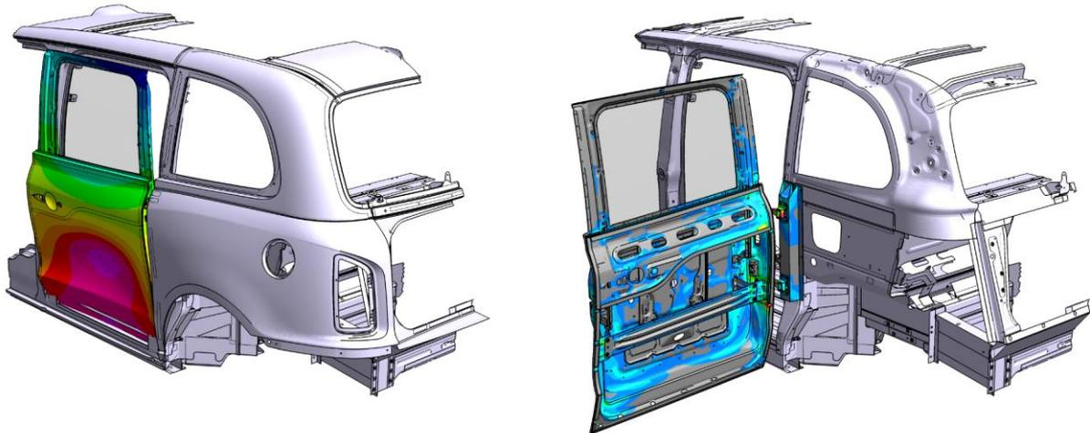
Fig.21: Rear door trimmed normal modes analysis (left) and open drop-off abuse case (right)
