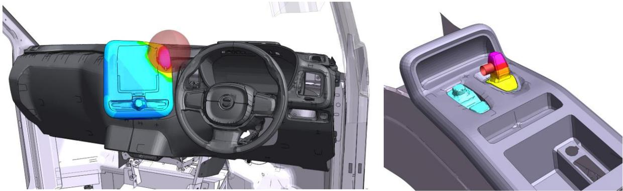
Fig. 18: ECE R21 Interior Head Impact to the Driver's Touchscreen (left) and Abuse loading to the gear selector (right)
