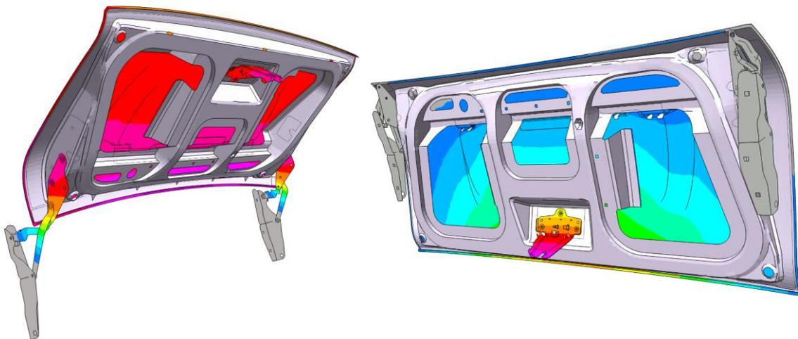
Fig.22: Trunk Lid in Open Lateral Abuse Case (left) and Closed Latch Loading (right)
