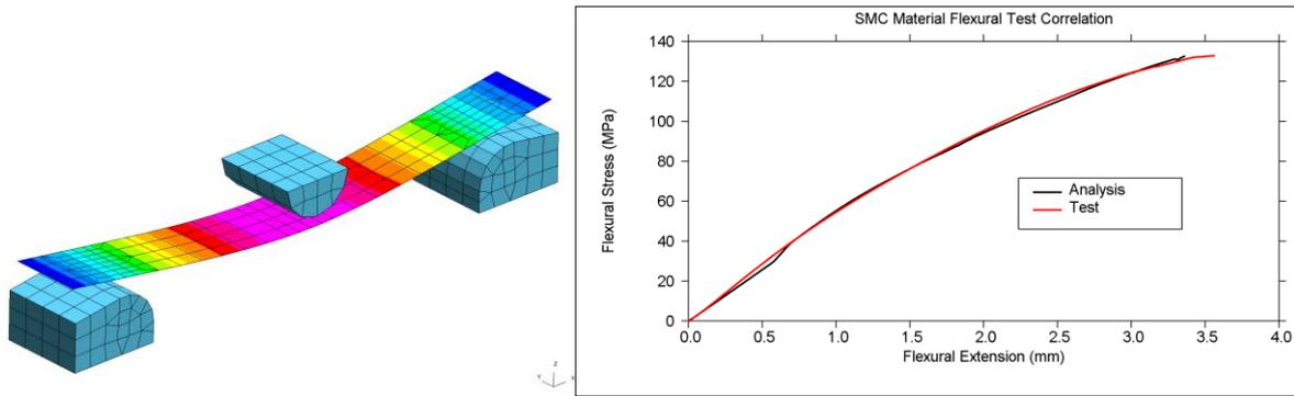
Fig.20: SMC flexural test model (left) and correlation of flexural response to test (right)
