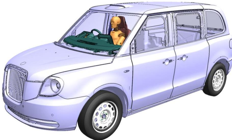
Fig.5: TX Finite Element Model
