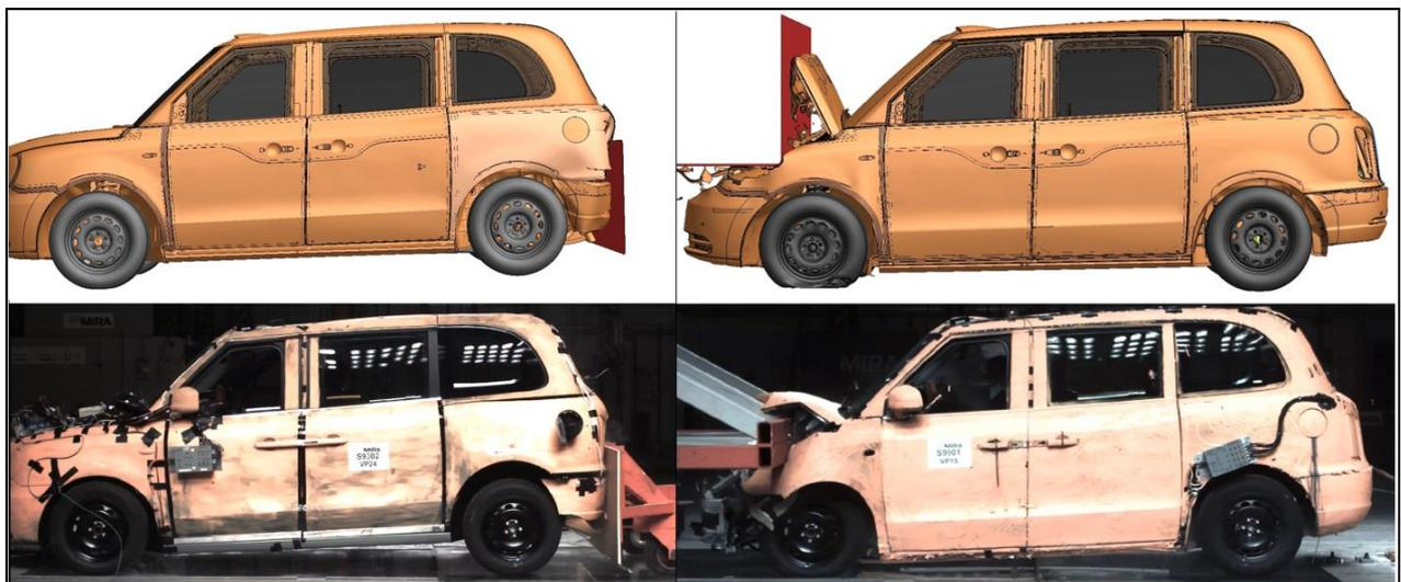
Fig.7: Comparison of Test and CAE; Rear Impact & Front Under-run
