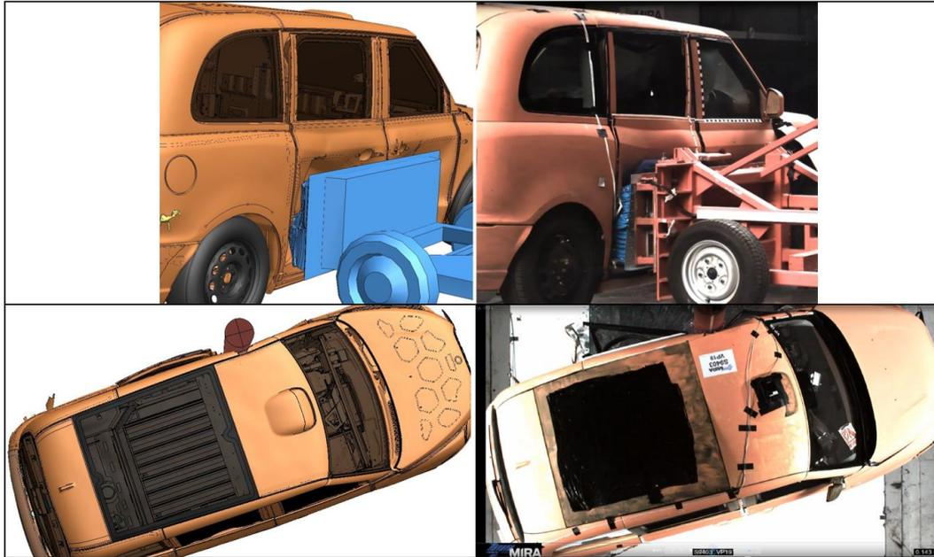
Fig.8: Comparison of Test and CAE; Side Barrier Impact & Pole Impact
