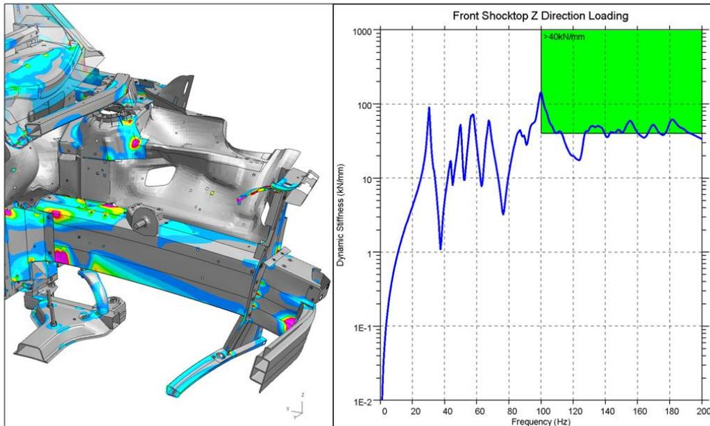
Fig. 16: Dynamic Stiffness of Front Suspension Mount
