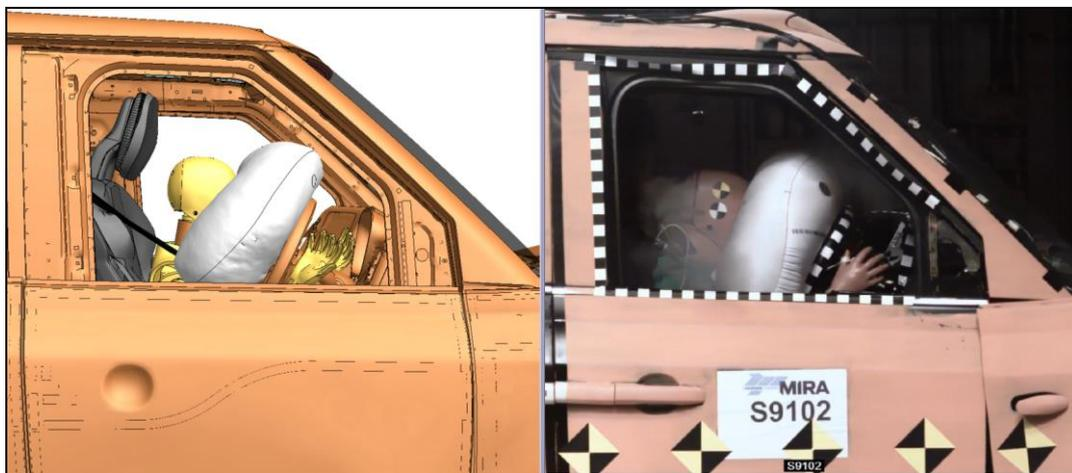
Fig.9: Front Impact with Small Female ATD, CAE & Test
