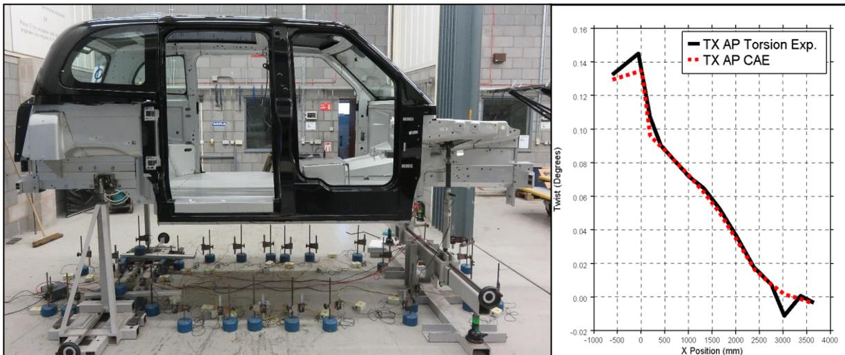
Fig. 15: BIW Static Torsion Test and Comparison with CAE
