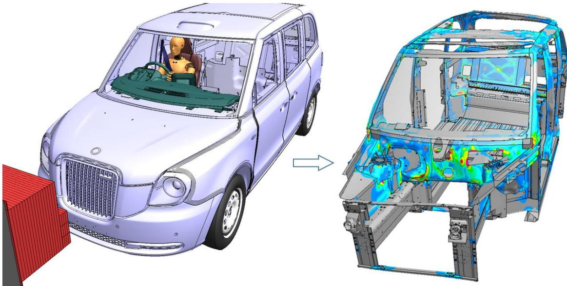
Fig. 14: Modular Model Approach and Typical Stiffness Analysis Output
