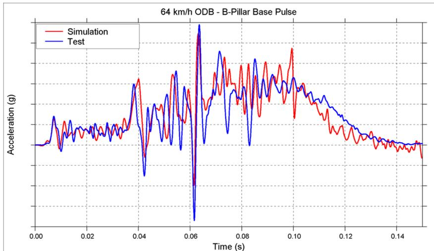
Fig.6: Example of Acceleration Time History Comparison for 64 km/h ODB Impact
