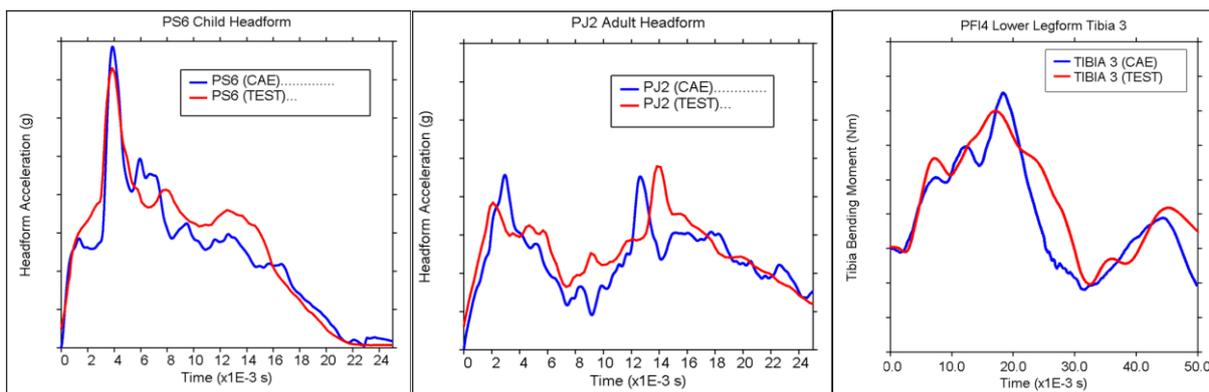
Fig.26: CAE to Test correlation for example Child Headform (left), Adult Headform (centre) and Lower Legform (right)
