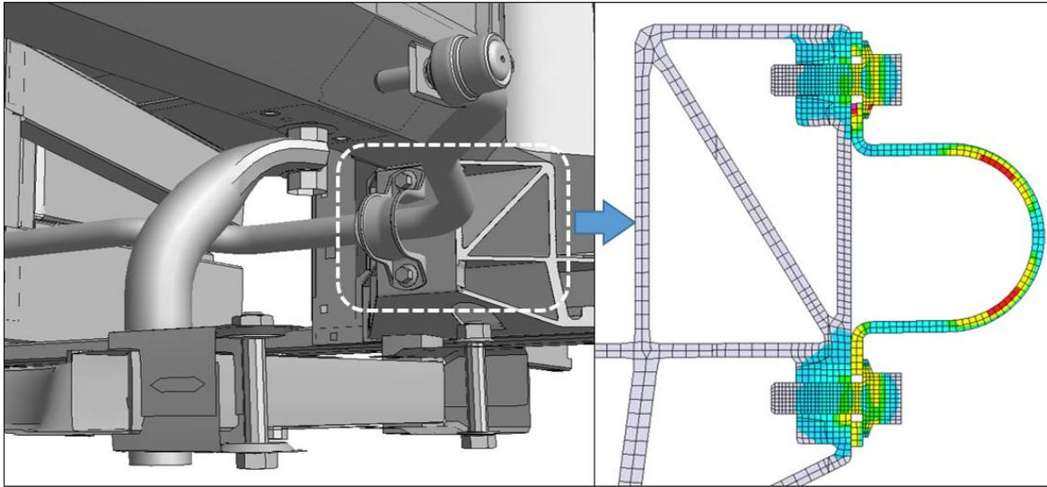
Fig.17: Detailed Model of Chassis System
