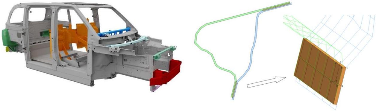
Fig.12: TX Bonded Aluminium BIW, Fig.2 - Detail of Solid Elements used for Adhesive
