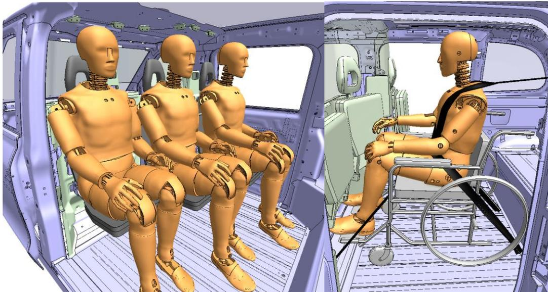
Fig.10: Second Row Occupant Model, Fig.11 Model of Occupant in Wheelchair
