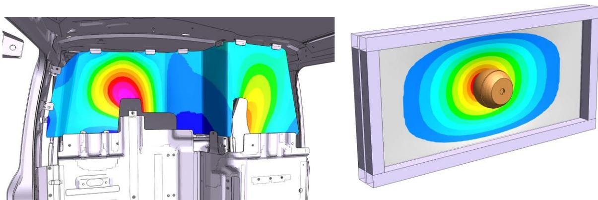
Fig. 19: Normal Modes Analysis (left) and ECE R43 Head Impact (right) to the Central Divider
