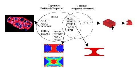
Figure 5. Genesis Topology and Topometry Designable Elements
