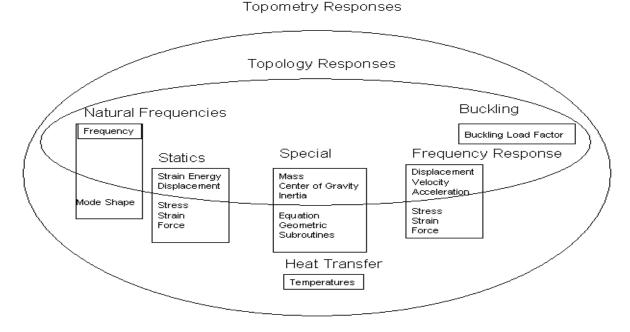
Figure 6. Types of Responses Available for Topology and Topometry Optimization
