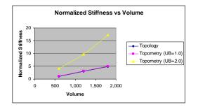
Figure 14. Normalized Stiffness for Different Volume Constraints
