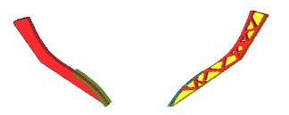
Figure 7. Topology Optimization. Initial and Final Designs
