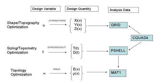
Figure 1. Optimization Types of Shell Elements
