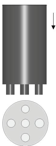
Direct extrusion, Punch speed 4mm/s
