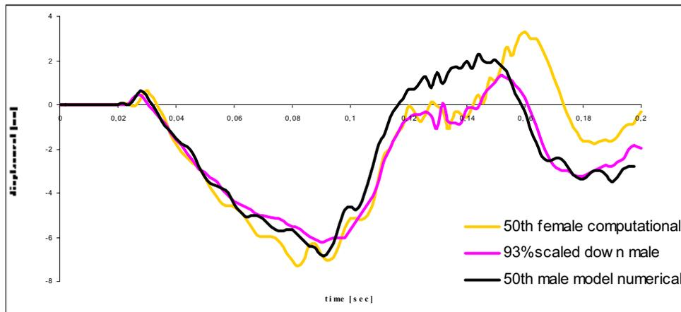
**Figure 6 C5 horizontal displacement relative to C6**
