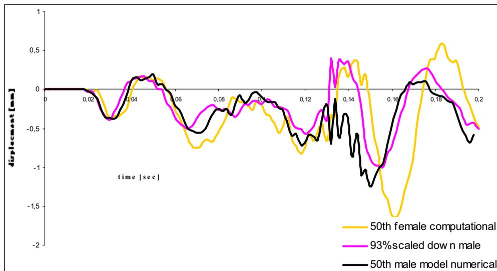
**Figure 7 C5 vertical displacement relative to C6**
