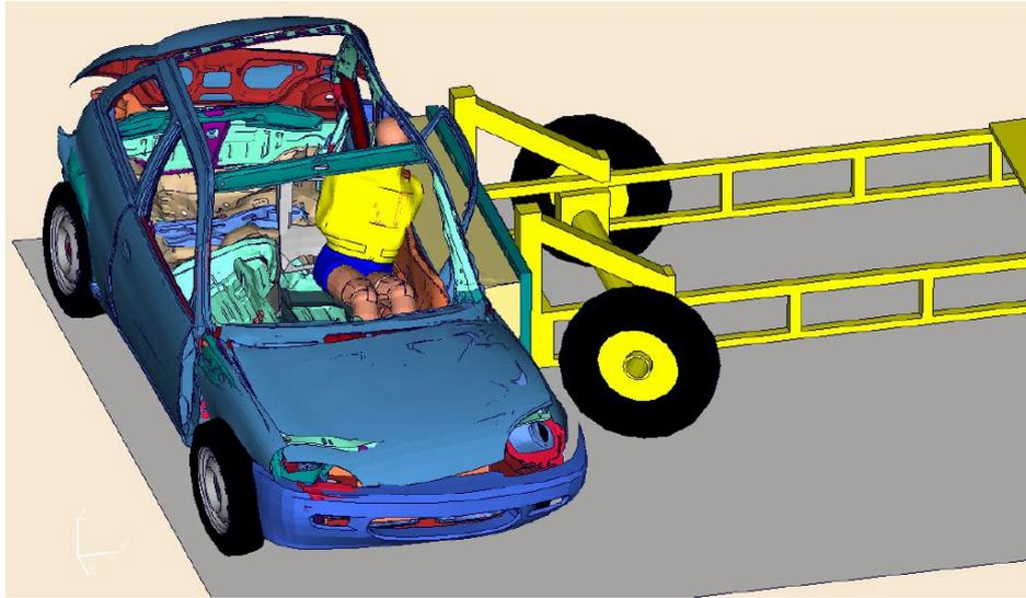
*LS-DYNA Vehicle & Barrier model coupled to MADYMO FE US-SID model*
