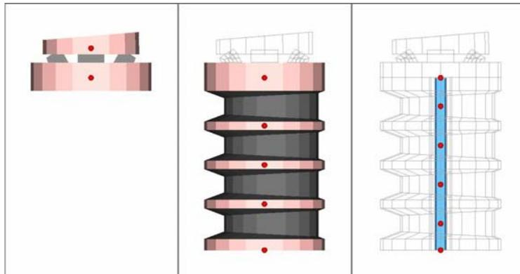
*Multibody neck sub models (Left: nodding joint, middle: nodding joint and neck-column without neck cable, right: complete neck including the neck-cable)*
