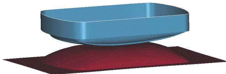
**Figure 2:** Simulation of the pre-forming operation and the resultant formed bubble of material
