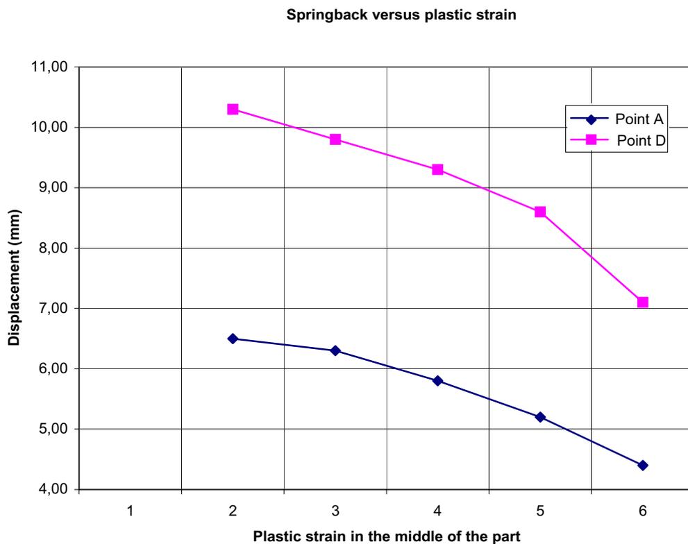
**Figure 7:** Spring-back tendency in connection with different plastic strain rates
