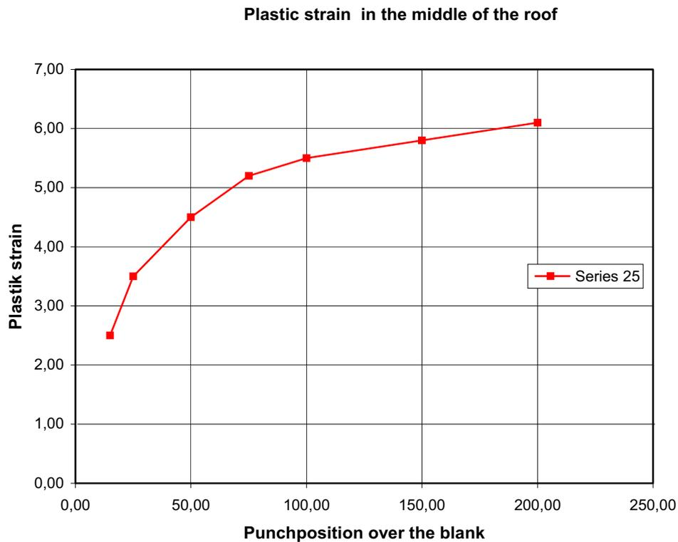
**Figure 4** Diagram of the plastic strain in the middle of the roof ( y-axis ) in correlation to the punch position ( x- axis)
