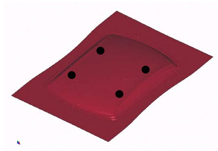
**Figure 5:** The roof component with the black spots showing the support in the simulation
