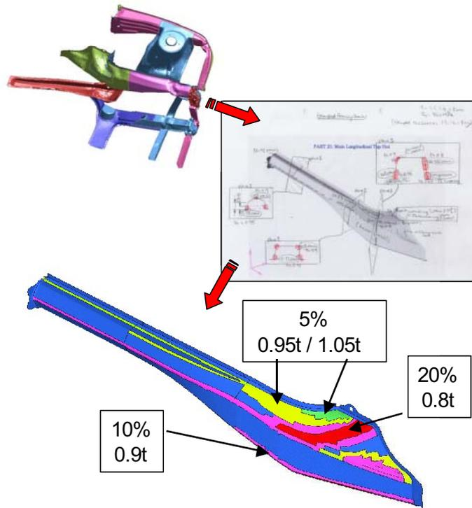
**Figure 6** Estimated Zones of Forming Strain
