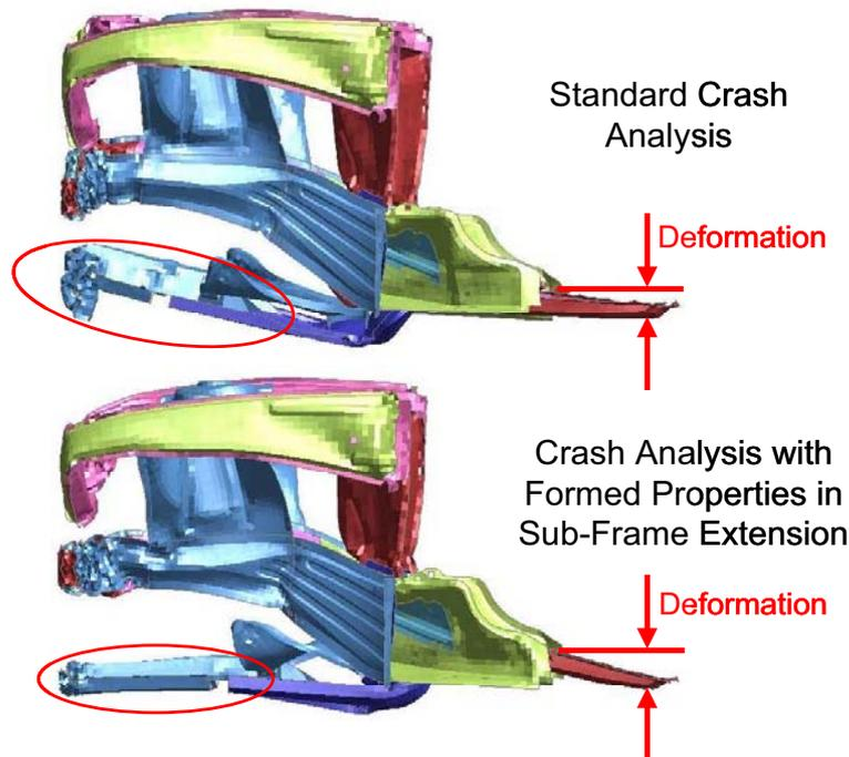
**Figure 5** Differences in Crash Performance Due to Forming in Full Vehicle Model
