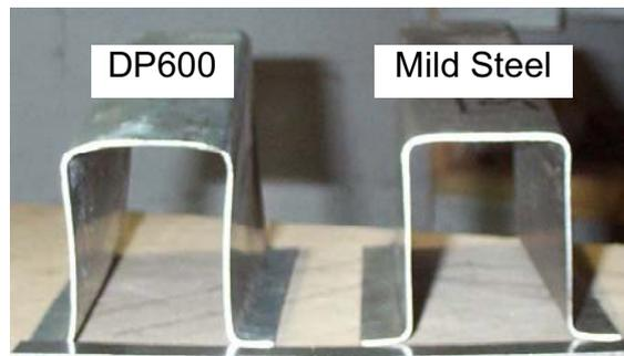
Figure 3 Component Shape After Forming
