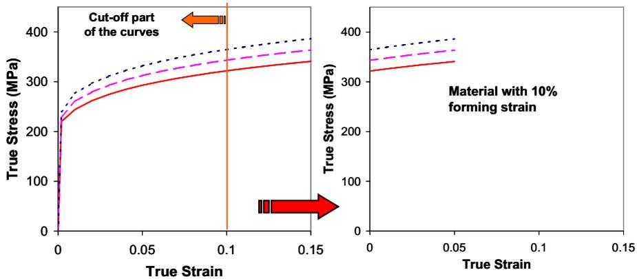
**Figure 7** Left-Shift of Material Strain Rate Curves
