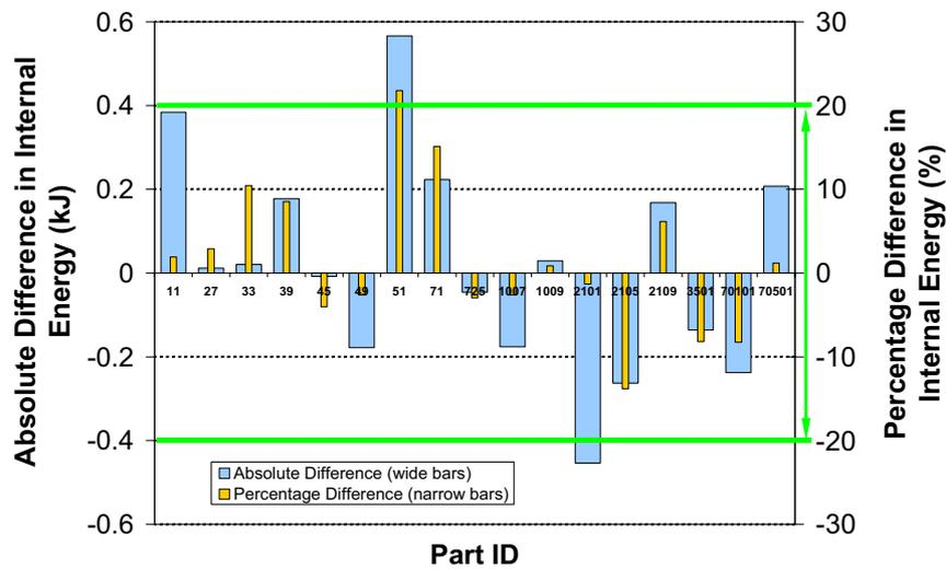
Figure 9 Comparisons of Internal Energies in Individual Parts for Approximate and Full F2C Analyses
