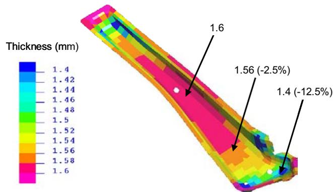
Figure 2 Material Thickness Change After Stamping
