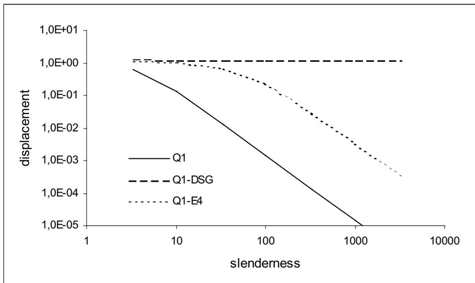
Figure 7 Bending of curved beam, curvature thickness locking (trapezoidal locking)
