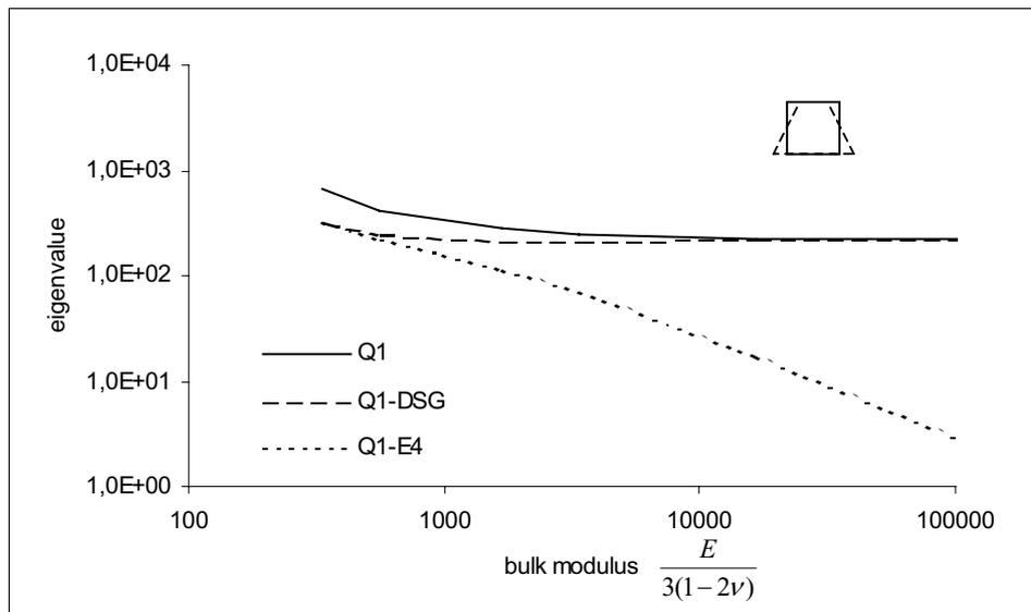
**Figure 5** Eigenvalue analyses of element stiffness matrices, volumetric locking
