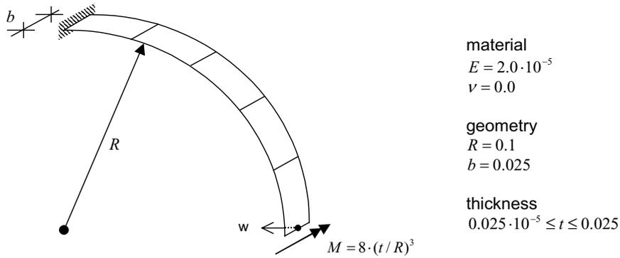
**Figure 7** Bending of cylindrical shell, problem setup
