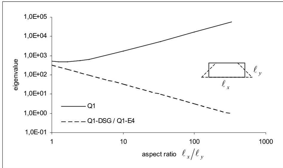
**Figure 4** Eigenvalue analyses of element stiffness matrices, shear locking
