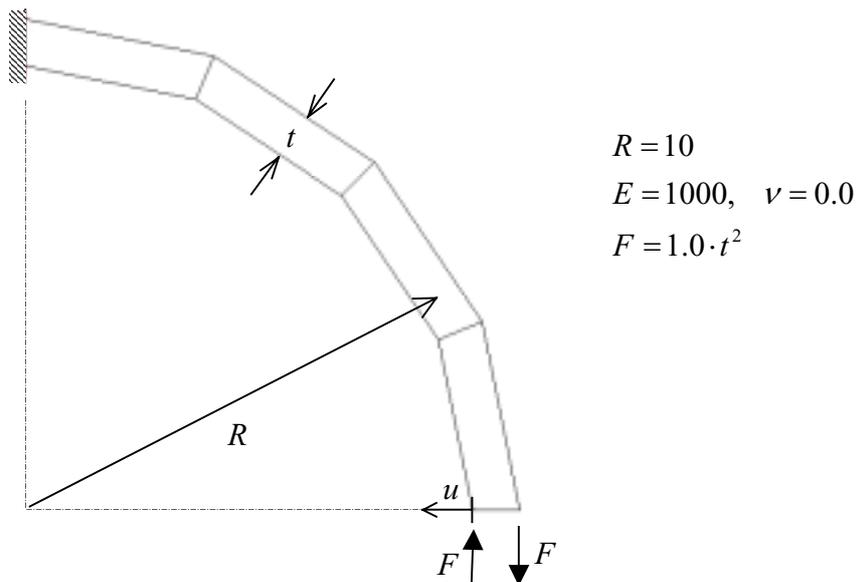
Figure 6 Bending of curved beam, problem setup
