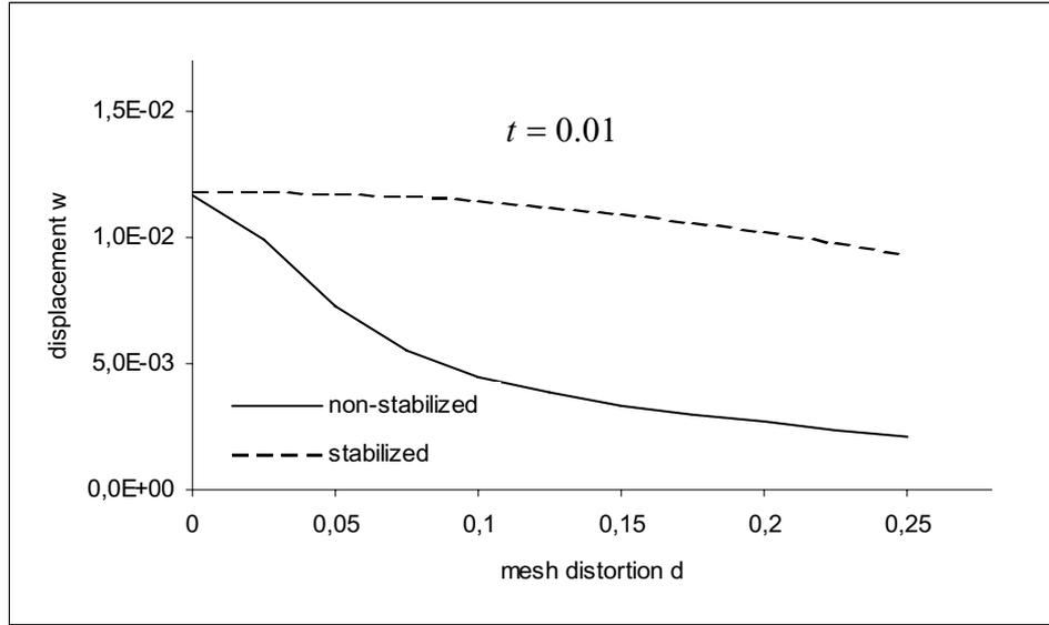
**Figure 3** Distortion sensitivity, constant thickness – varying mesh distortion
