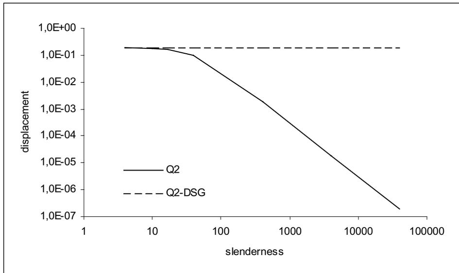
**Figure 8** Bending of cylindrical shell, membrane locking
