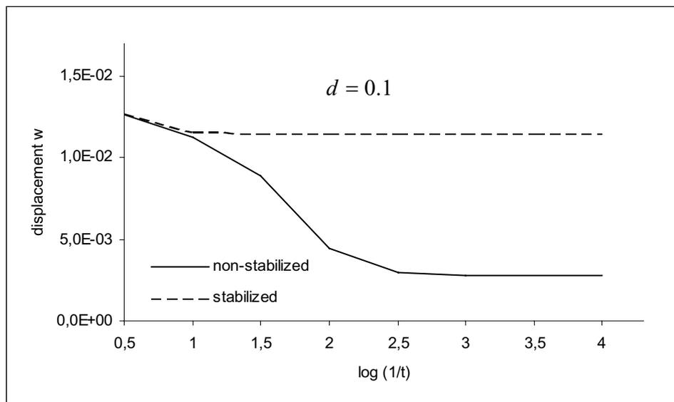
**Figure 2** Distortion sensitivity, constant mesh – varying thickness
