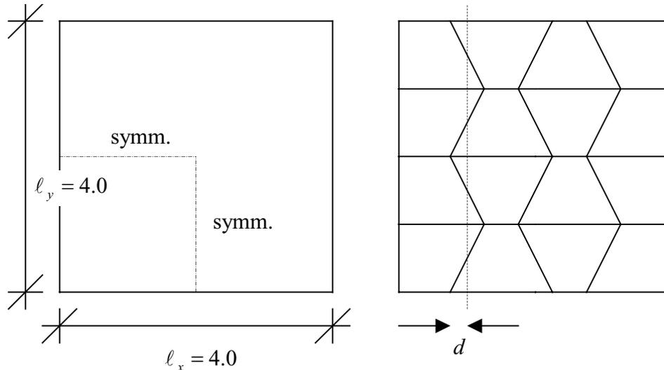
**Figure 1** Sensitivity to mesh distortion, problem setup
