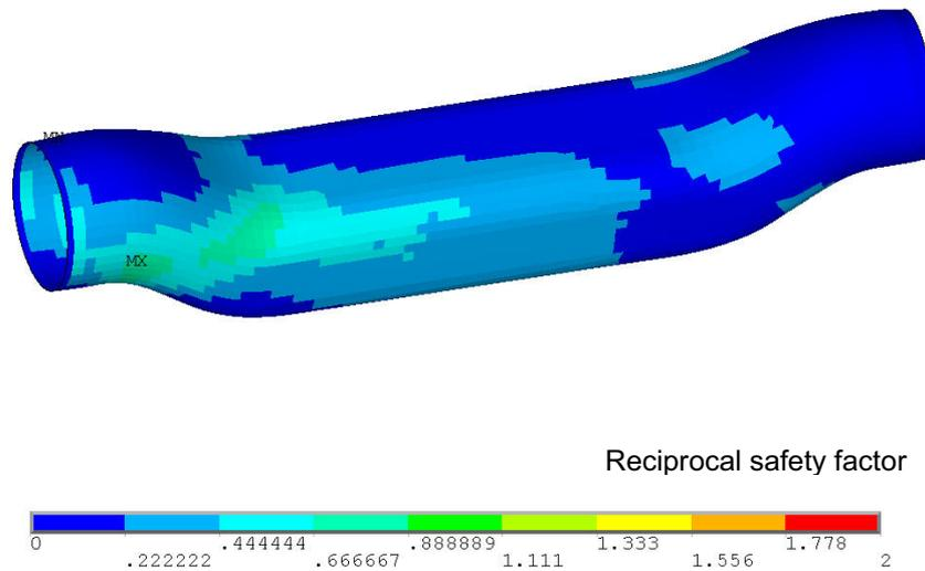
**Figure 11:** The result of the ANSYS® calculation with the related strain hardening
