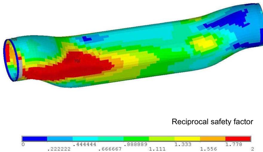
**Figure 12:** The result of the ANSYS® calculation without strain hardening
