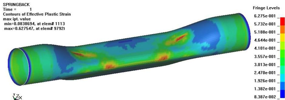
**Figure 8:** Contours of Effective Plastic Strain after the springback calculation
