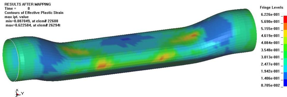
**Figure 9:** Contours of Effective Plastic Strain after the mapping
