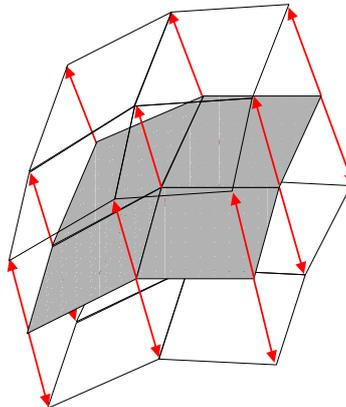
**Figure 2** A diagrammatic representation of the calculation of the inner and outer (or upper and lower) point cloud
