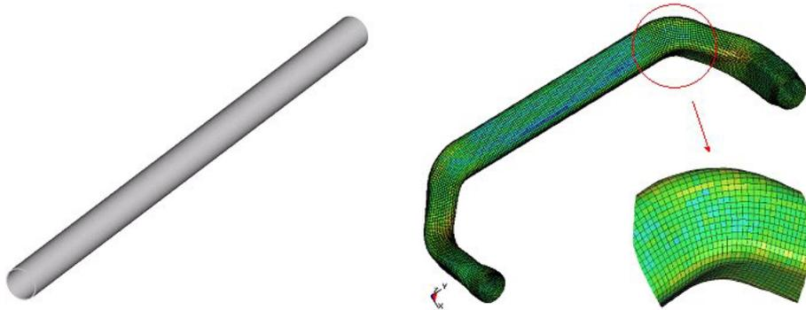
**Figure 5:** The unformed tube (left) and the result of the forming simulation (right)
