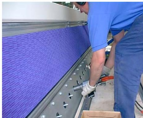
**Fig 3**    Bodyside Huckbolted™ joint
