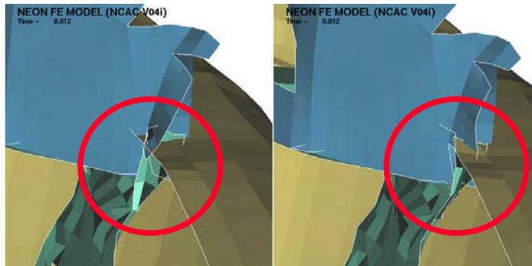
**Figure 6:** Behaviour of Neon part 377 in two different simulation runs at 12 ms.
