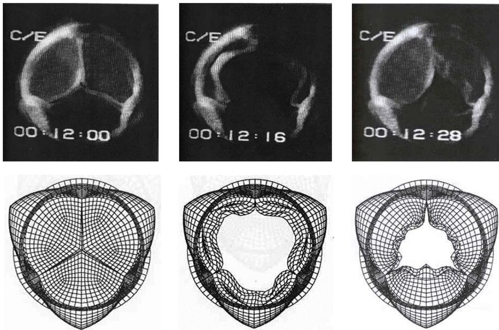
Figure 10 – Views, from the downstream or aorta, of the displacements of the valve leaflets at selected instants in the cardiac cycle. Data from the simulation (*below*) reflect that shown in pictures from a pulse duplicator study of a porcine valve (*above*). The pictures and plots show the opening and subsequent closing of the valve in nominally 40ms increments.
