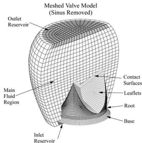
Figure 8. The aortic valve model, showing the inlet and outlet reservoirs. The Control volume allows for lateral flow as the sinuses (not shown) and aortic wall expand and contract.
