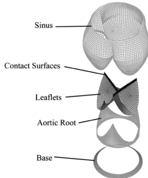
Figure 6 – Schematic diagram of the idealisation of the aortic valve and its surrounding structure showing parameters used to define the geometry.
