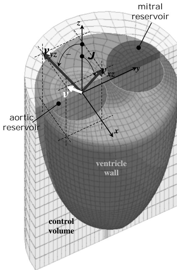
Figure 4 – Section through the ventricular flow domain showing shell elements of the ventricle model contained within it, and the alignment of the inlet and outlet reservoirs.
