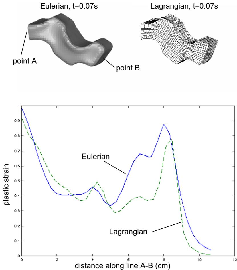
Figure 5. Effective plastic strain level at  $t=0.07s$
