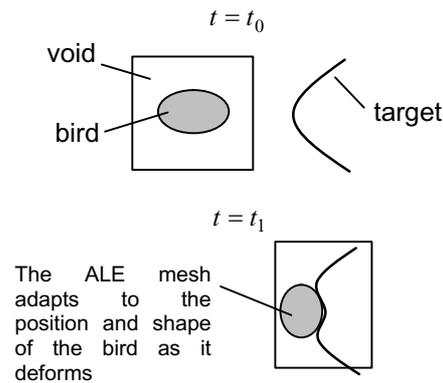
Figure 1. Moving ALE-mesh in impact simulation
