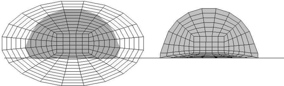
Figure 8. Material contours of impacting balls.
