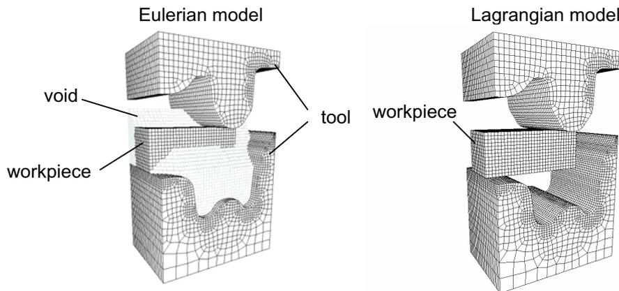
Figure 3. Eulerian and Lagrangian forging models
