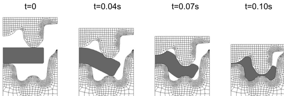
Figure 4. Cross section of Eulerian work-piece at different stages of the process
