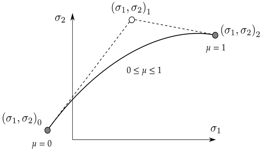
Figure M136-1. Bézier interpolation curve.
