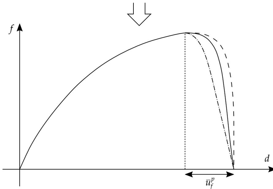
**Figure 2-2.** Top plot illustrates plastic displacement at failure as a function of damage for a given triaxiality for DETYP = 0 and  $\alpha = 0$ . The different curves illustrate different possible types of post-instability characteristics. The bottom plot illustrates qualitatively how these curves may interact in a tension test.  $d$  is the displacement and  $f$  is the force.
