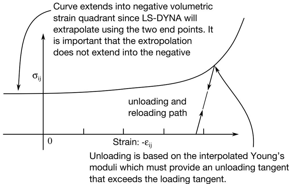
**Figure M26-1.** Stress quantity versus volumetric strain. Note that the “yield stress” at a volumetric strain of zero is non-zero. In the load curve definition, see \*DEFINE\_CURVE, the “time” value is the volumetric strain and the “function” value is the yield stress.
