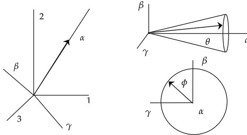
**Figure M266-1.** The plot on the left relates the global coordinates (1, 2, 3) to the local coordinates  $(\alpha, \beta, \gamma)$ , selected so the mean fiber direction in the reference configuration is align with the  $\alpha$ -axis. The plots on the right show how the unit vector for a specific fiber within the fiber distribution of a 3D tissue is oriented with respect to the mean fiber direction via angles  $\theta$  and  $\phi$ .
