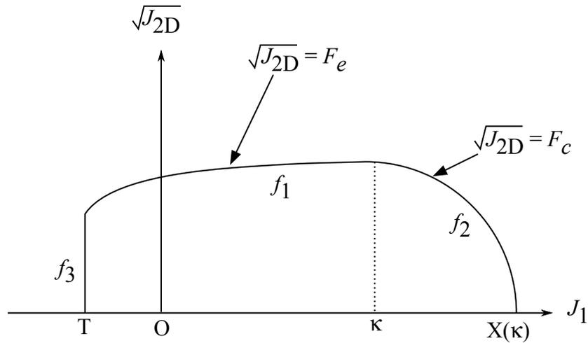
**Figure M25-1.** The yield surface of the two-invariant cap model in pressure  $\sqrt{J_{2D}} - J_1$  space. Surface  $f_1$  is the failure envelope,  $f_2$  is the cap surface, and  $f_3$  is the tension cutoff.
