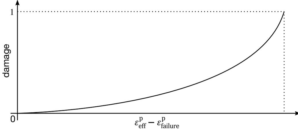
**Figure M81-2.** A nonlinear damage curve is optional. Note that the origin of the curve is at (0,0). The nonlinear damage curve is useful for controlling the softening behavior after the failure strain EPPF is reached.
