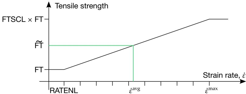
**Figure M280-2.** Modified tensile strength of elements neighboring an element that has at least one failed integration point as a function of strain rate when  $\text{RATENL} > 0.0$ .  $\dot{\epsilon}^{\max} = 10^9 \times \text{RATENL}$ .
