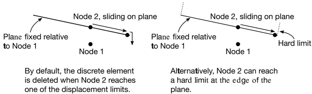
**Figure M205-1.** Illustration of the two different actions that can be applied to the element when Node 2 reaches the edge of the plane. The left schematic depicts the default behavior in which the element is deleted when Node 2 reaches the edge. The right image illustrates Node 2 reaching a hard limit. When it reaches this limit, a contact force is applied.
