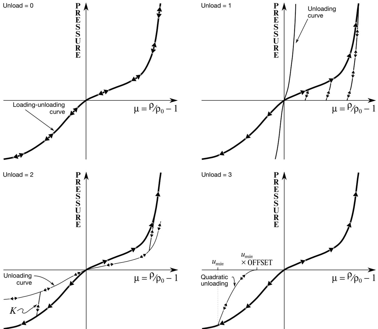
Figure EOS15-1. Load and unloading behavior.
