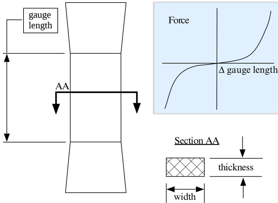
Figure M27-1. Uniaxial specimen for experimental data
