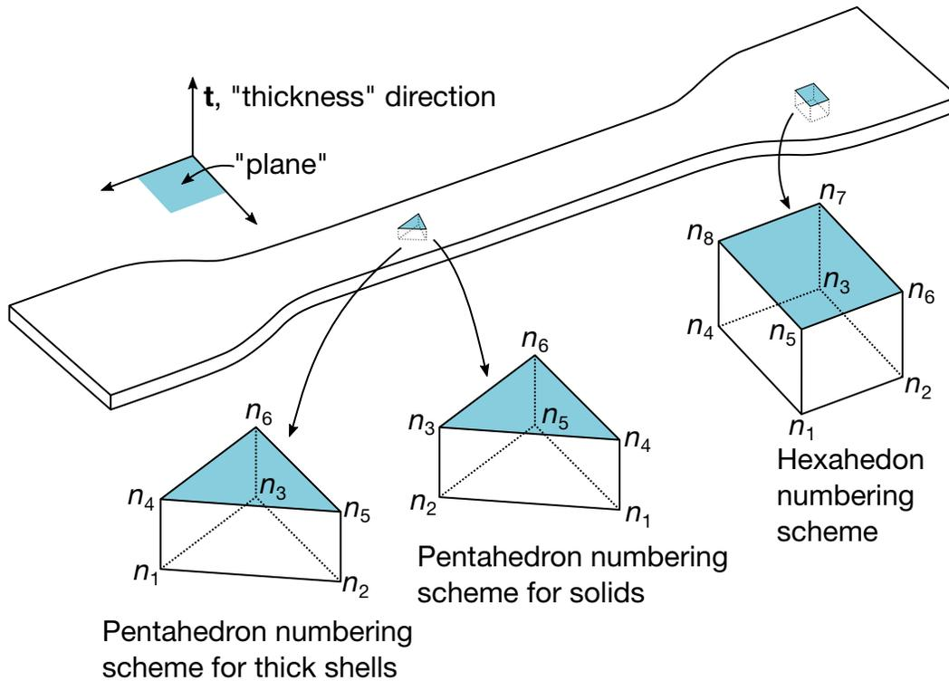
**Figure 2-1.** Solid and thick shell elements must be oriented in a part in a specific way when using MSFLD or FLD (DITYP = 2 or 3). This figure illustrates the required element numbering scheme and the thickness direction,  $t$ .
