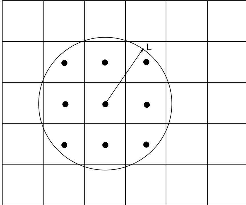
**Figure 2-6.** Here  $\dot{f}_r$  and  $x_r$  are respectively the nonlocal rate of increase of damage and the center of the element  $e_r$ , and  $\dot{f}_{local}^i$ ,  $V_i$  and  $y_i$  are respectively the local rate of increase of damage, the volume and the center of element  $e_i$ .
