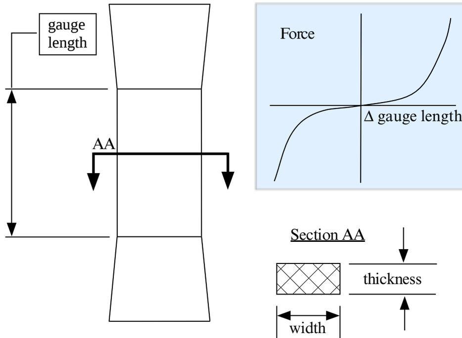
**Figure M218-1.** Uniaxial specimen for experimental data
