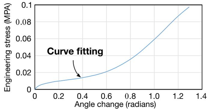
**Figure M293-3.** An example of the angle change-engineering stress curve from the bias-extension test. The curve fit for this example is  $y = -0.29x^6 + 1.09x^5 - 1.68x^4 + 1.37x^3 - 0.56x^2 + 0.12x$ . For this example curve the inputs into LS-DYNA are  $G121 = -0.29$ ,  $G122 = 1.09$ ,  $G123 = -1.68$ ,  $G124 = 1.37$ ,  $G125 = -0.56$ , and  $G126 = -0.12$  [3].
