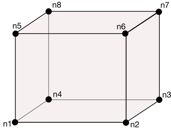
**Figure M100-1.** A solid element used as spot weld is shown. When resultant based failure is used orientation is very important. Nodes n1 - n4 attach to the lower shell mid-surface and nodes n5 - n8 attach to the upper shell mid-surface. The resultant forces and moments are computed based on the assumption that the brick element is properly oriented.
