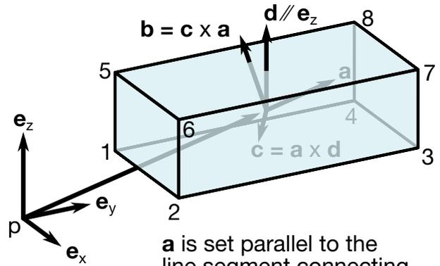
**a** is set parallel to the line segment connecting **p** to the element center.
