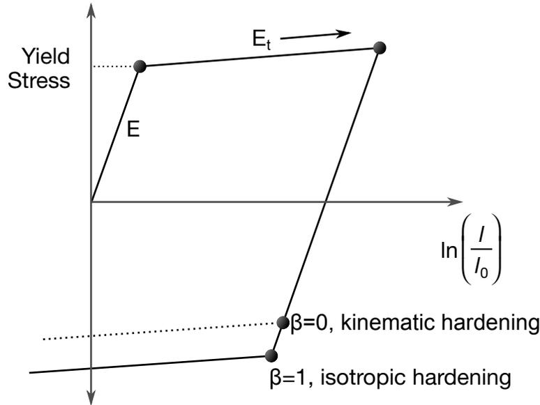
**Figure M3-1.** Elastic-plastic behavior with kinematic and isotropic hardening where  $l_0$  and  $l$  are undeformed and deformed lengths of uniaxial tension specimen.  $E_t$  is the slope of the bilinear stress strain curve.
