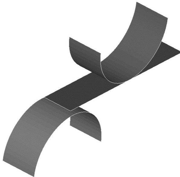
**Figure C.2** Shell mesh for the user element test.
