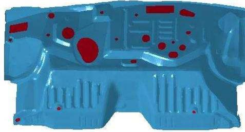
Trimmed-out Holes Filled with LS-PrePost
