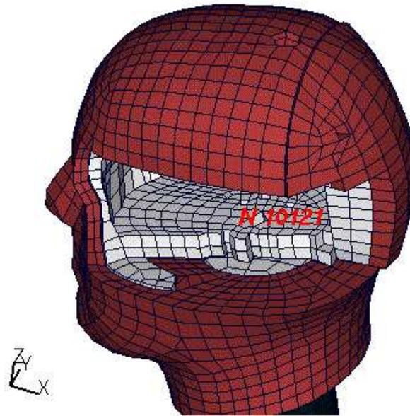
Fig. 4: nodes for extracting head accelerations
