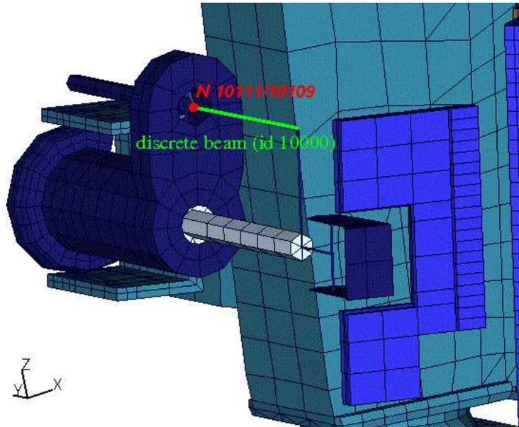
Fig. 5: nodes for extracting rib intrusion
