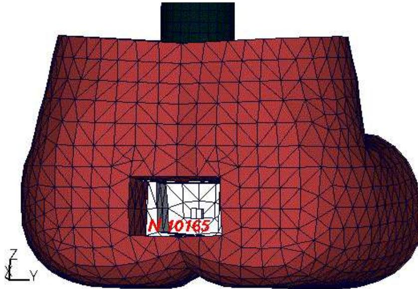
Fig. 3: nodes for extracting pelvis accelerations
