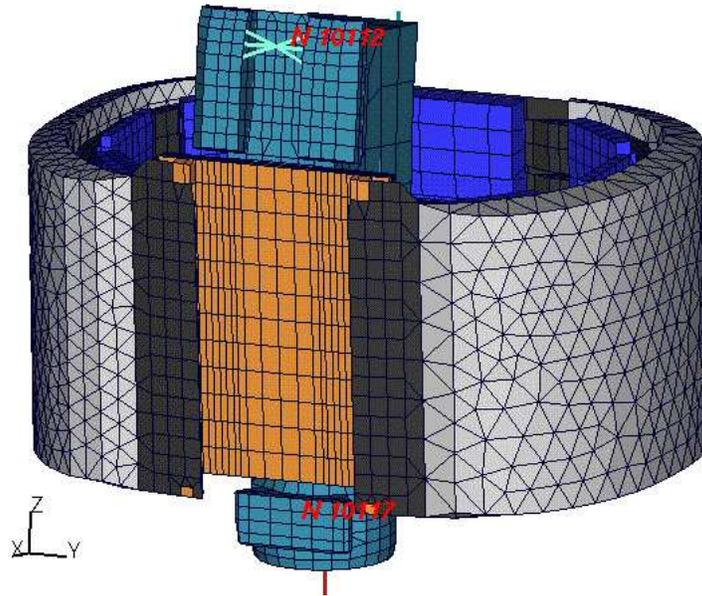
Fig. 2: nodes for extracting spine accelerations
