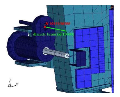
Fig. 5: nodes for extracting rib intrusion
