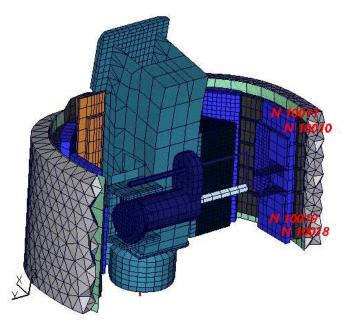
Fig. 1: nodes for extracting rib accelerations
