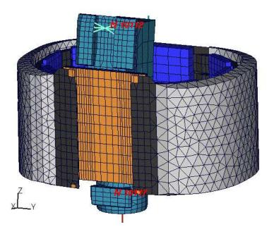
Fig. 2: nodes for extracting spine accelerations
