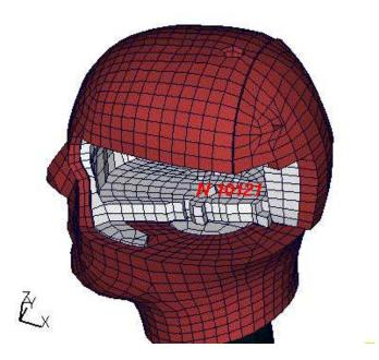
Fig. 4: nodes for extracting head accelerations
