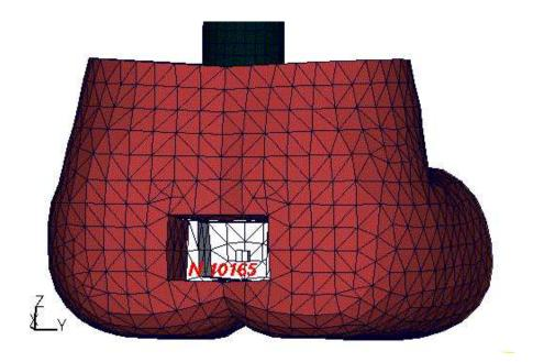
Fig. 3: nodes for extracting pelvis accelerations
