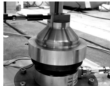
Figure 1: Thrust measurement test setup
