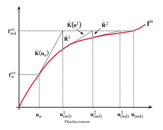
Figure 1 – This figure shows the progress of nonlinear equilibrium iterations advancing a solution from time "n" to time "n+1". Superscripts on displacement variables indicate nonlinear iterations.
