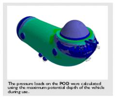
Naturally, most of the pressure management effort goes into protecting the pilot. DeepFlight Aviator uses a rigid cast aluminum body. More than anything else, the pod resembles a bent cocoon. It is a cylinder tapering from 26 inches in diameter at the pilot's shoulder level to 18 inches at the feet.
