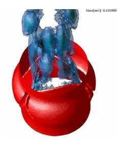
The above is an FSI problem of a opening valve and the flow is shown and maximum aperture when the flow rate peaks. In both cases the turbulence was modeled using a LES approach.
