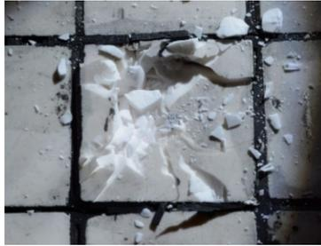
*Fig.2: Impact damage example: 48x48x65 mm ceramic on 9 mm rubber after 500 J impact*
