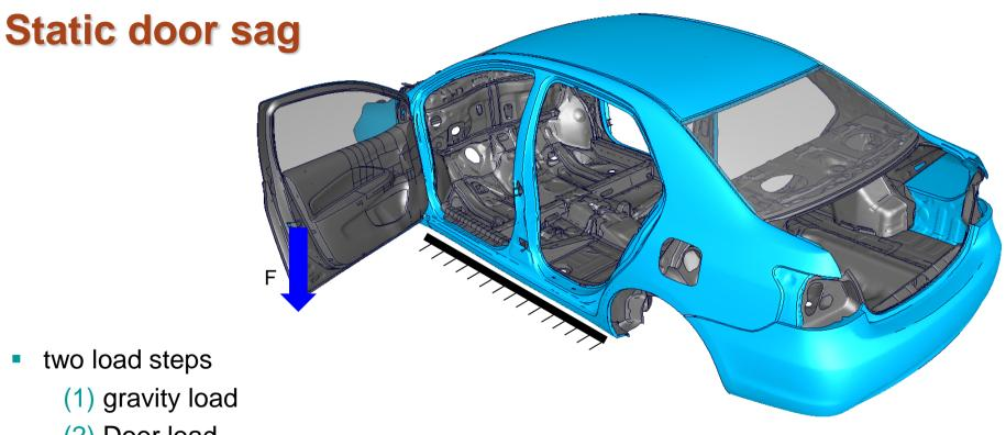
(1) gravity load (2) Door load
