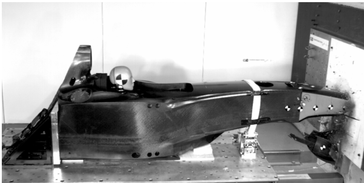
Figure 3: Frontal impact crash test setup
