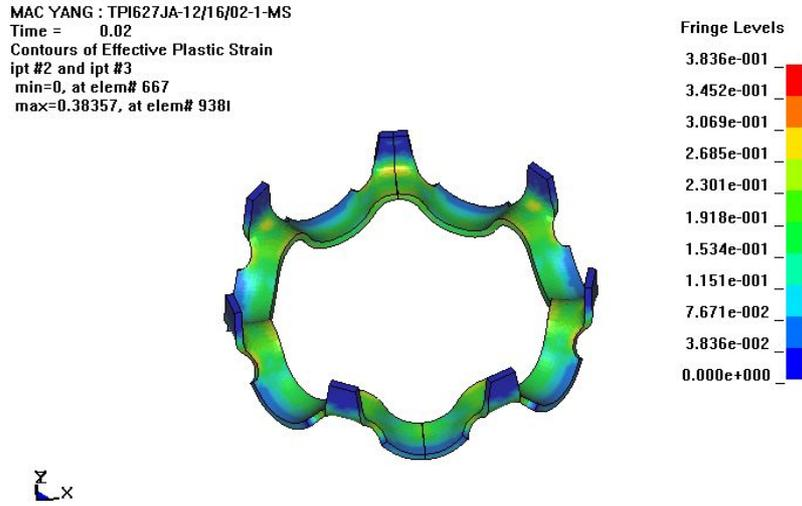
**Figure 9** The plastic strain distribution of finished form stage.
