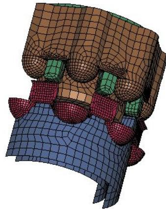
**Figure 7** The finished-form stage Punch, Holder and Die mesh model.
