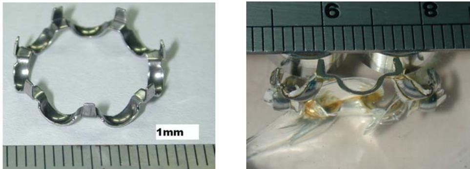
**Figure 11** The final stamping part and its cross section at the cage.
