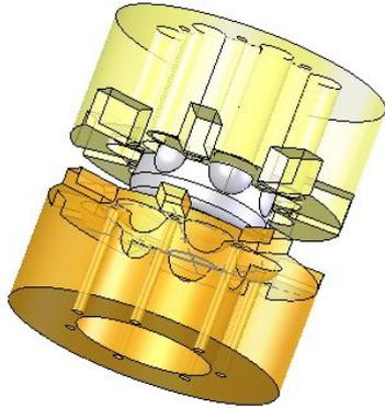
**Figure 6** The finished-form stage Punch, Holder and Die CAD model.
