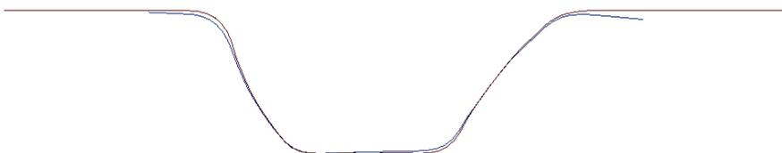
**Figure 8** Section 3, desired shape of the sheet and shape after first springback iteration
