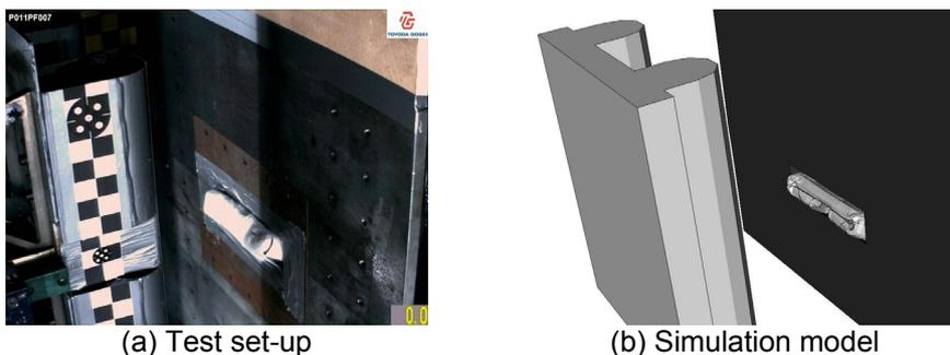
Figure 8: Combined knee-tibia impactor test set-up and simulation model
