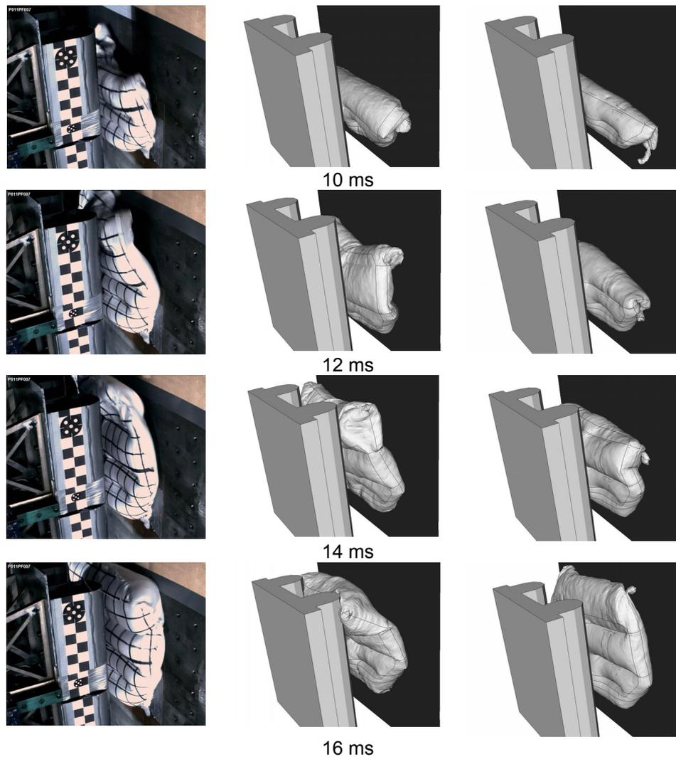
Figure 13: PKAB early inflation animation test versus CVM and CPM time history – m1 impactor
