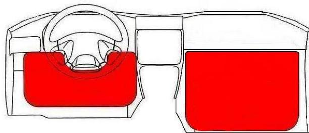
*Figure 2: Driver knee airbag (DKAB) and passenger knee airbag (PKAB) application*
