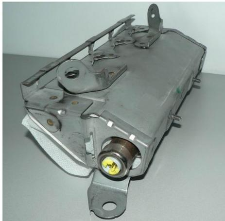
Figure 4: Emphasised cylindrical inflator location in the real DKAB module with container
