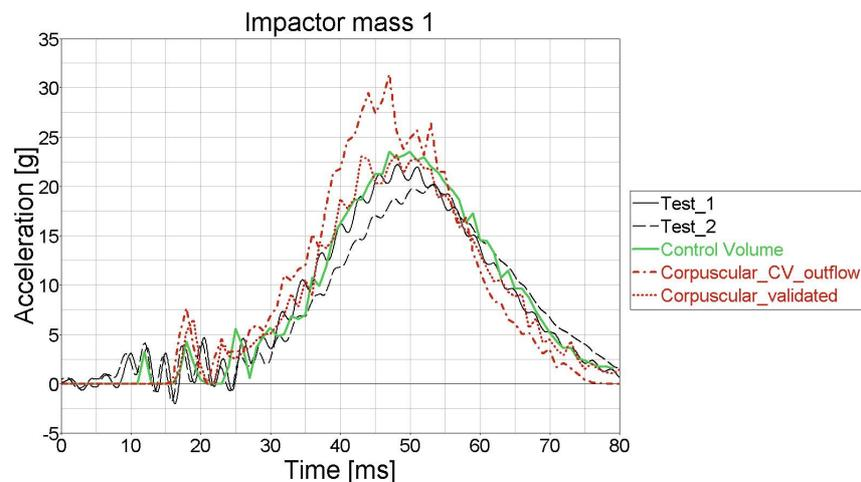
Figure 15: DKAB CPM outflow effect for the impactor (m1) test acceleration time history
