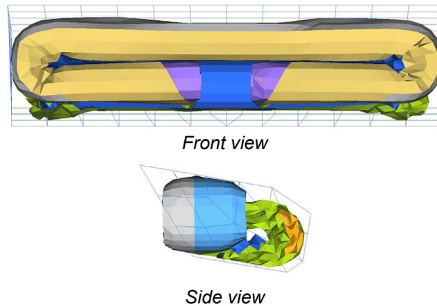
Figure 7: Folded PKAB FE package model (relaxed FE mesh) – front and side view
