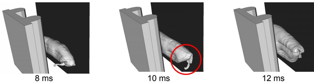
Figure 19: PKAB cushion twisting observed during CPM unfolding
