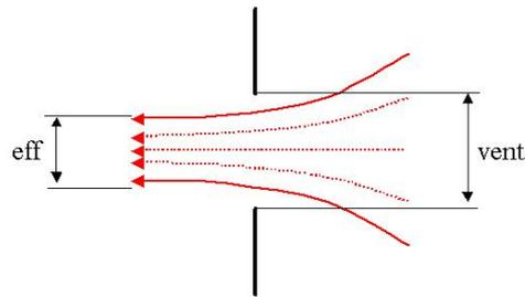
Figure 14: Effective outflow area decrease through an orifice indicated by streamlines
