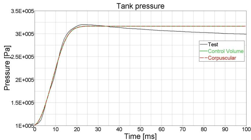
Figure 9: Tank pressure time history, CVM versus CPM result
