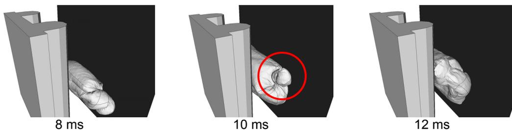
Figure 18: DKAB cushion twisting observed during CVM unfolding
