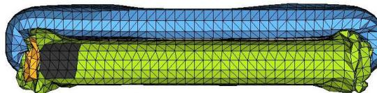
Figure 6: DKAB vent hole modelling for CPM simulation
