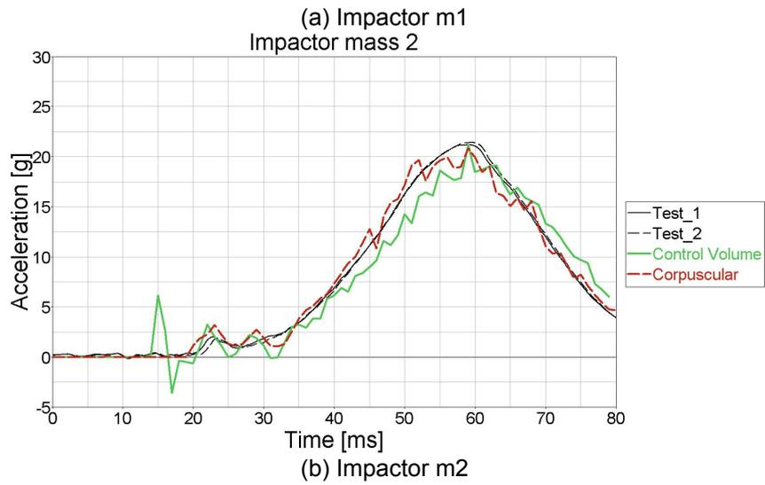
Figure 12: PKAB dynamic impactor acceleration prediction
