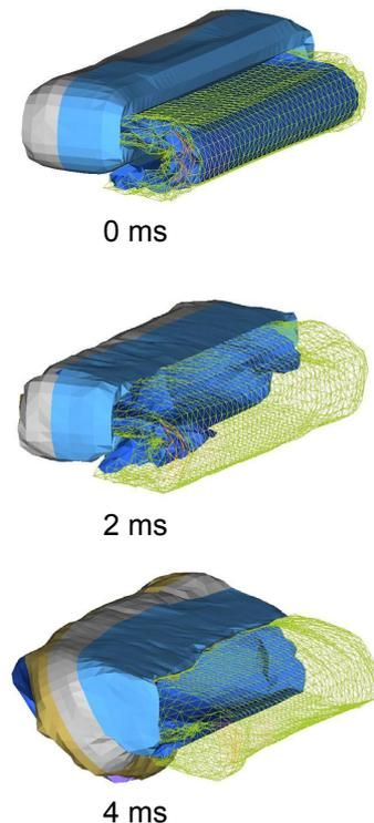
Figure 17: Initial gas flow into the folded package – DKAB model
