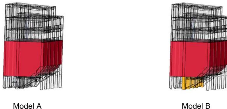
Figure 4: Discretization approaches, Model A - silo as non eroding part, Model B - silo and columns in the middle axis as non eroding parts
