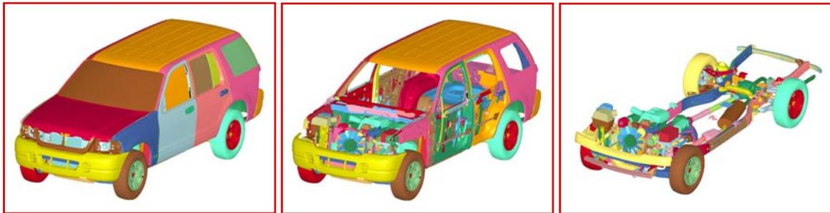
Figure 2: Finite Element Model of the Exemplar Vehicle
