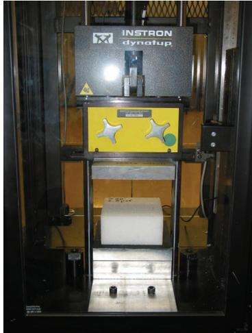
Figure 4a: Drop tower test set-up.
