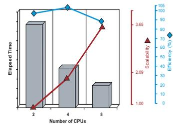
Figure 1: Scalability of the three-car-crash benchmark run on a single Sun Fire X4600 server with eight 3.0 GHz Opteron processors
