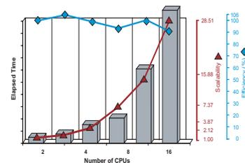
Figure 2: Scalability of the FLUENT CFD benchmark run on a Sun Blade 8000 modular system with four 4-processor Sun Blade X8400 server modules
