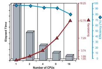
Figure 3: Scalability of STAR-CD turbulent flow around an A-class car, by a cluster of Sun Fire X2100 servers with Opteron processors (gigabit Ethernet)
