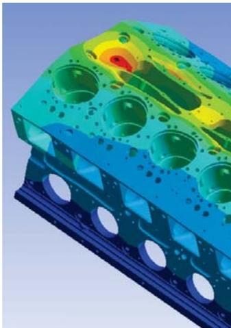
Deformation contours on an engine block, courtesy of ANSYS, Inc.
