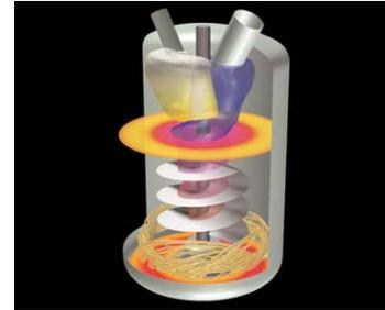
Crutcher mixer CFD simulation using FLUENT, FIELDVIEW image courtesy of Intelligent Light
