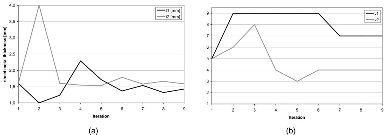
**Figure 6:** Optimization with LS-OPT: Variables (a)  $t_1$ ,  $t_2$  and (b)  $v_1$ ,  $v_2$  for calculated successive optima
