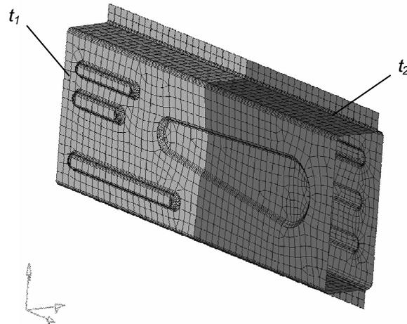
**Figure 4:** Simulation model of a longitudinal member made of Tailored Blanks
