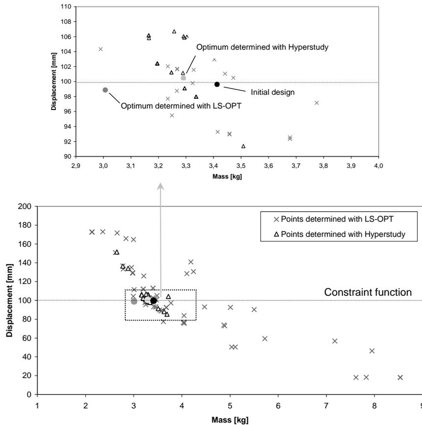
**Figure 10:** Mass vs. displacement for all with LS-OPT and Hyperstudy calculated designs and determined optima
