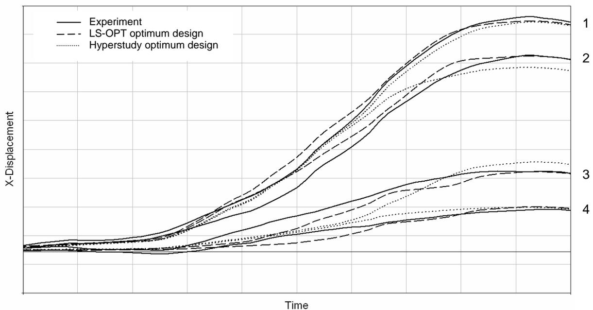
**Figure 12:** Result of the optimization with LS-OPT and Hyperstudy: x-Displacement of the corners of the plate over simulation time
