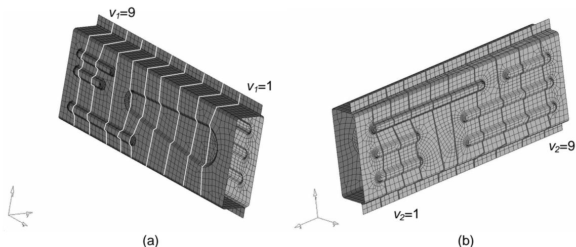
**Figure 5:** Defined discrete positions for the weld seam; (a)  $v_1$  for the inner shell and (b)  $v_2$  for the outer shell
