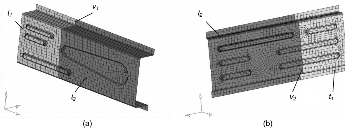
**Figure 9:** Optimum Design determined with Hyperstudy (a) inner shell (b) outer shell with  $t_1=1,37$  mm  $t_2=1,60$  mm  $v_1=7$   $v_2=7$  Mass=3,29 kg
