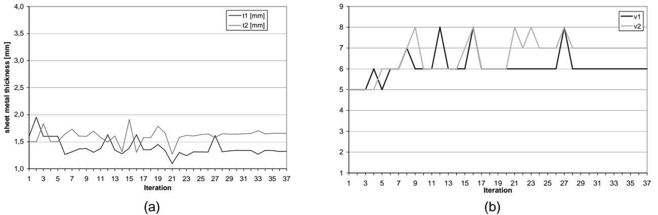
**Figure 8:** Optimization with Hyperstudy: Variation of variables (a)  $t_1$ ,  $t_2$  and (b)  $v_1$ ,  $v_2$  within the design space over number of iterations
