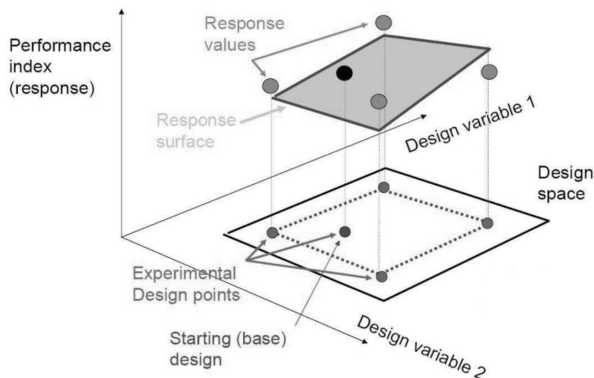
**Figure 1:** Principle of creating an approximation with Response Surface Methodology [2]
