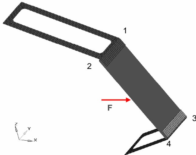
**Figure 11:** Simulation Model of the plate. The Movement of the plate is caused by the force  $F$  and is dependent on the sheet metal widths of the strips 1 - 4
