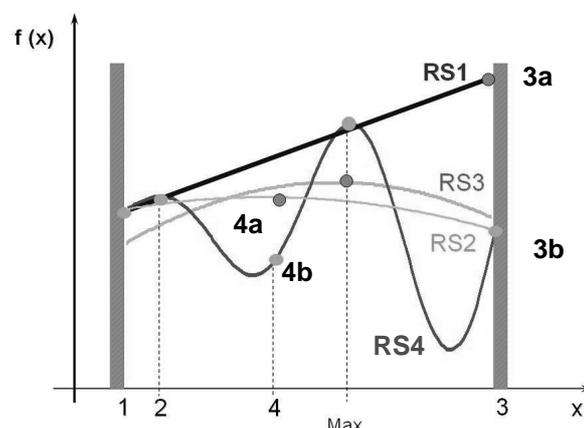
Figure 3: Principle of determining an optimum with the Sequential Response Surface method [4]
