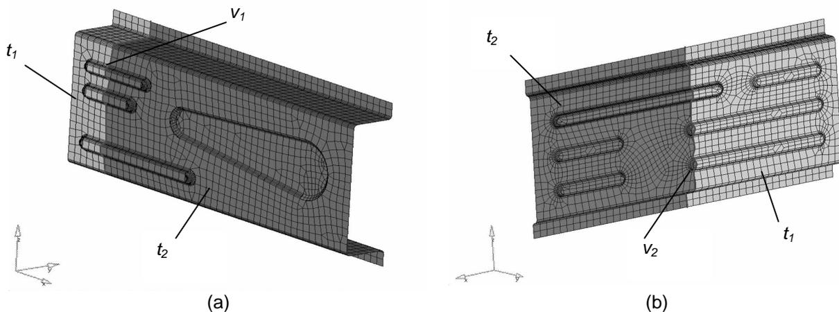
**Figure 7:** Optimum design determined with LS-OPT (a) inner shell (b) outer shell with  $t_1=1,02$  mm  $t_2=1,58$  mm  $v_1=9$   $v_2=4$  Mass=3,01 kg
