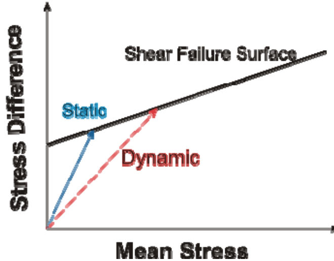
Figure 3 Schematic of static and dynamic, with inertial confinement, unconfined compression test.
