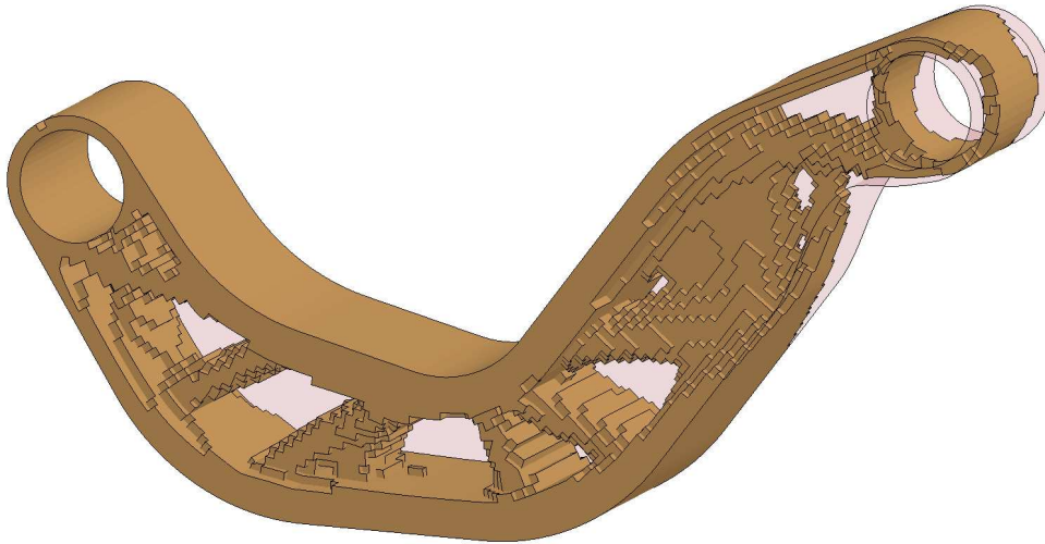
Figure 9: Final design for casting problem. The outline of the original design is also shown.
