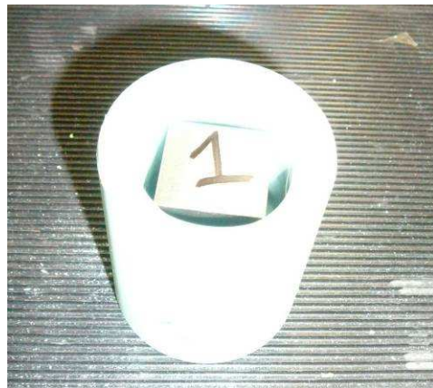
Figure 3 : Sabot and steel cube projectile used for the test
