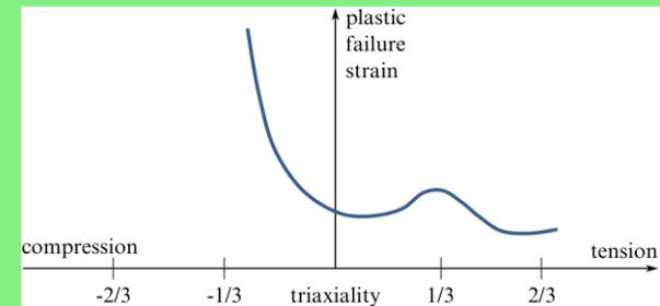
3D: add. lode-angle-dependency → failure surface
