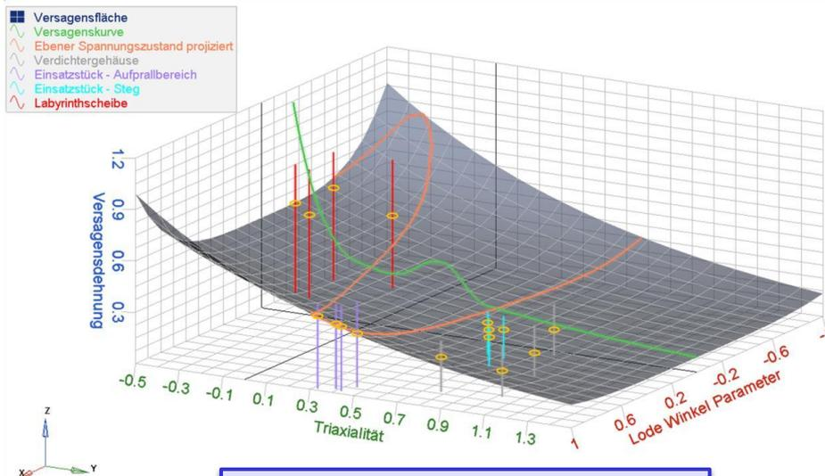
Lode angle parameter and triaxiality in the elements of failure
