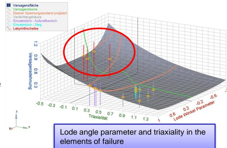
Lode angle parameter and triaxiality in the elements of failure
