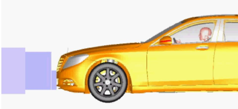
I: Integrated structure- and occupant simulation
