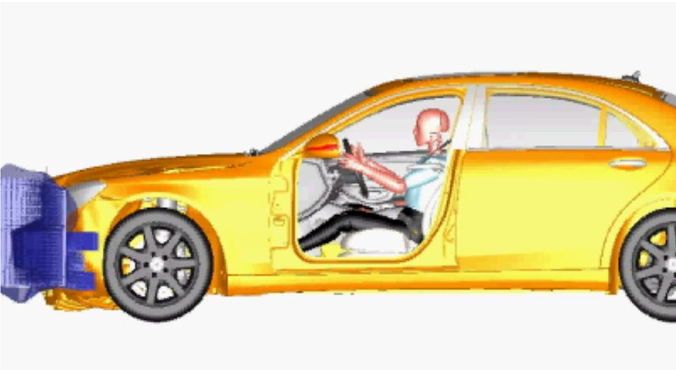
II: Model reduction to occupant cell (sled) model
