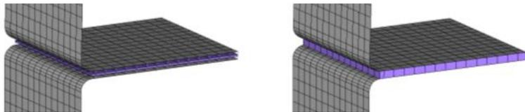
Adhesive modeling: real thickness/gap thickness
