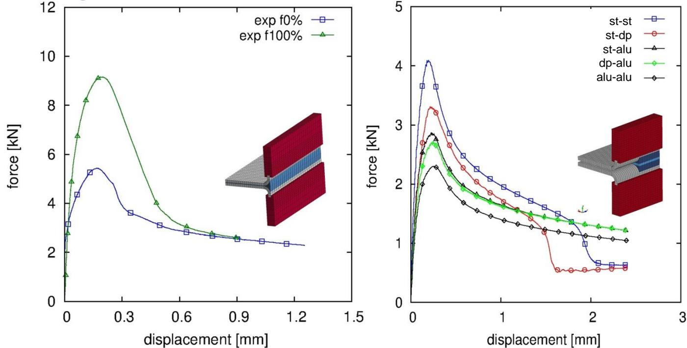
**➔ Gapfilling and substrate have substantially influence on the force maximum**
