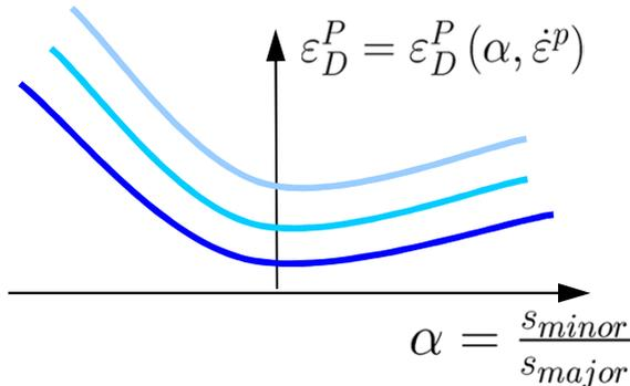
The MSFLD damage initiation criterion (DITYP=2) only considers the evolution of plastic strain if the pressure is negative (i.e., compressive stress states have no effect). The damage initiation variable is defined as
