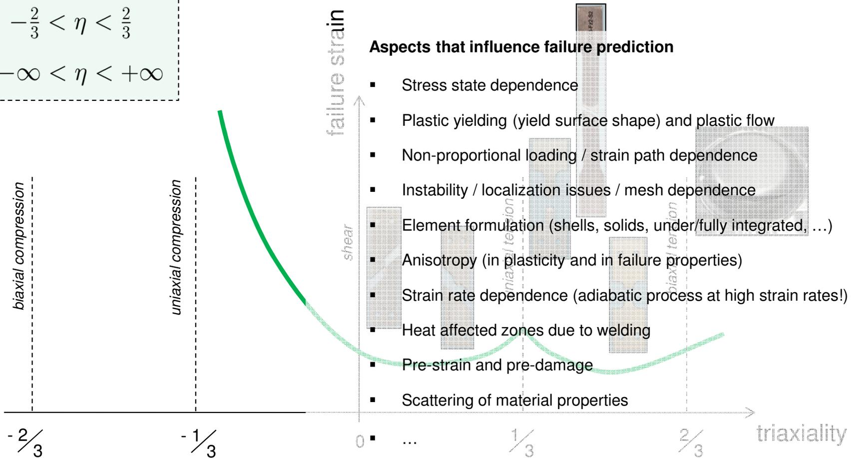
Suitable specimens are needed for the accurate calibration of material failure
