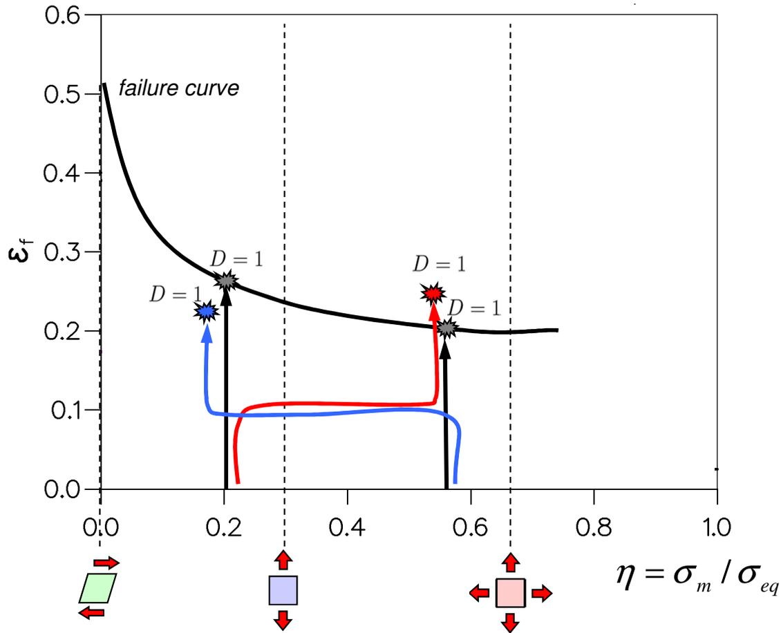
Damage is incrementally accumulated as a function of the plastic strain increment and of the failure curve. **Failure occurs when  $D = 1$ !**
