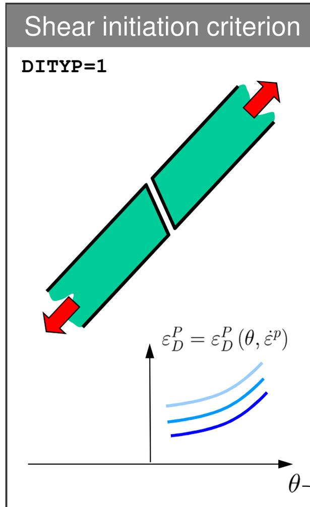
Accumulation of the damage initiation variable:
