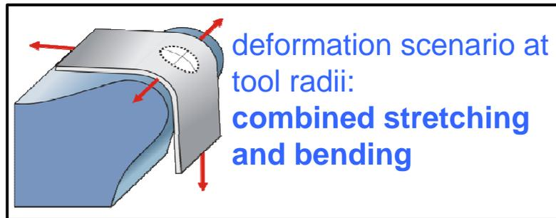
➔ conventional failure criteria fail to reliably predict forming limits if bending is involved
