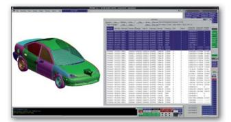
PRIMER has been specially and exclusively designed for LS-DYNA as an FE solver. In many cases, PRIMER is also applied to check LS-DYNA models for errors or to remove redundant entries that may cause problems. In addition, the program offers a range of special properties to model occupant safety simulations, such as dummy positioning, seat adjustment, seatbelt fitting, or airbag folding.
